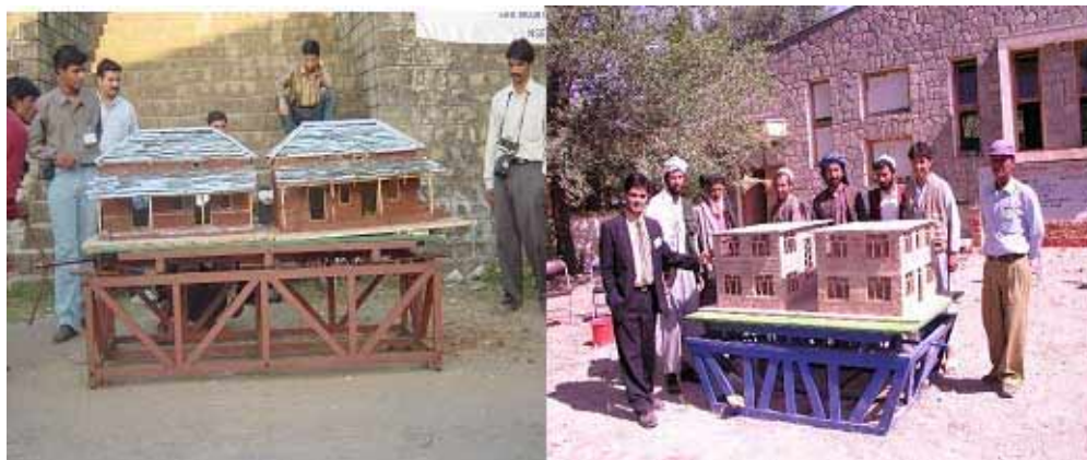
Figure 3. 1:10 scale shake table testing with rural construction in Northern India (Left) and Kabul, Afghanistan (Right). The photo in the right shows Nepalese mason and engineer with Afghani masons
