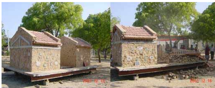
Figure 2. Shake table demonstration testing (building types: stone with mud mortar)
