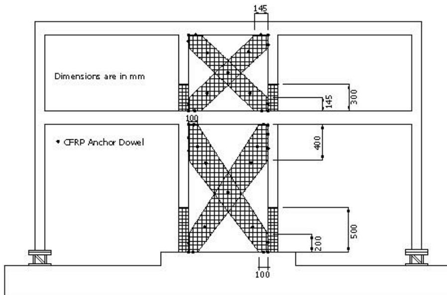
**Figure 4. Configuration of the CFRP and Location of Anchor Dowels**
