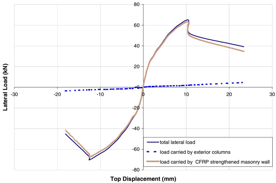
**Figure 10. Load Sharing Envelopes of the Members of Specimen S2**
