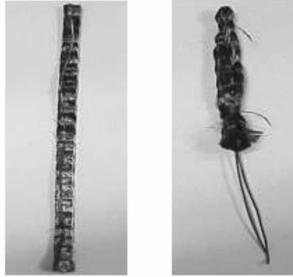
**Figure 5. Anchor Dowel in the Infill (Left), Anchor Dowel in the concrete members (Right)**
