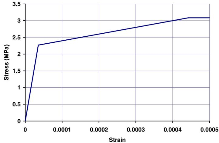
**Figure 14. Tension Strut Model for Composite Material**
