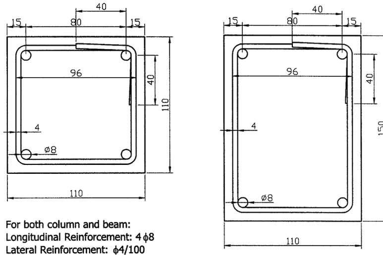
**Figure 2. Column and Beam Cross-Section**
