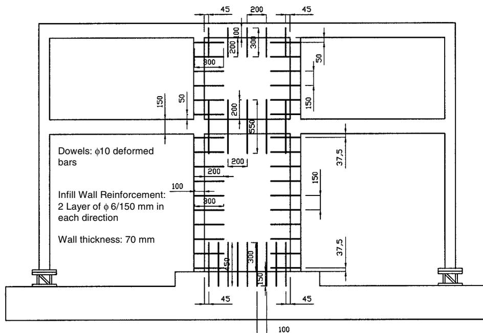
**Figure 3. Steel Anchor Dowels (All dimensions are in mm)**
