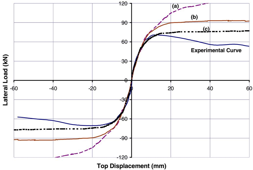
**Figure 11. Response Envelopes of Specimen S1**
