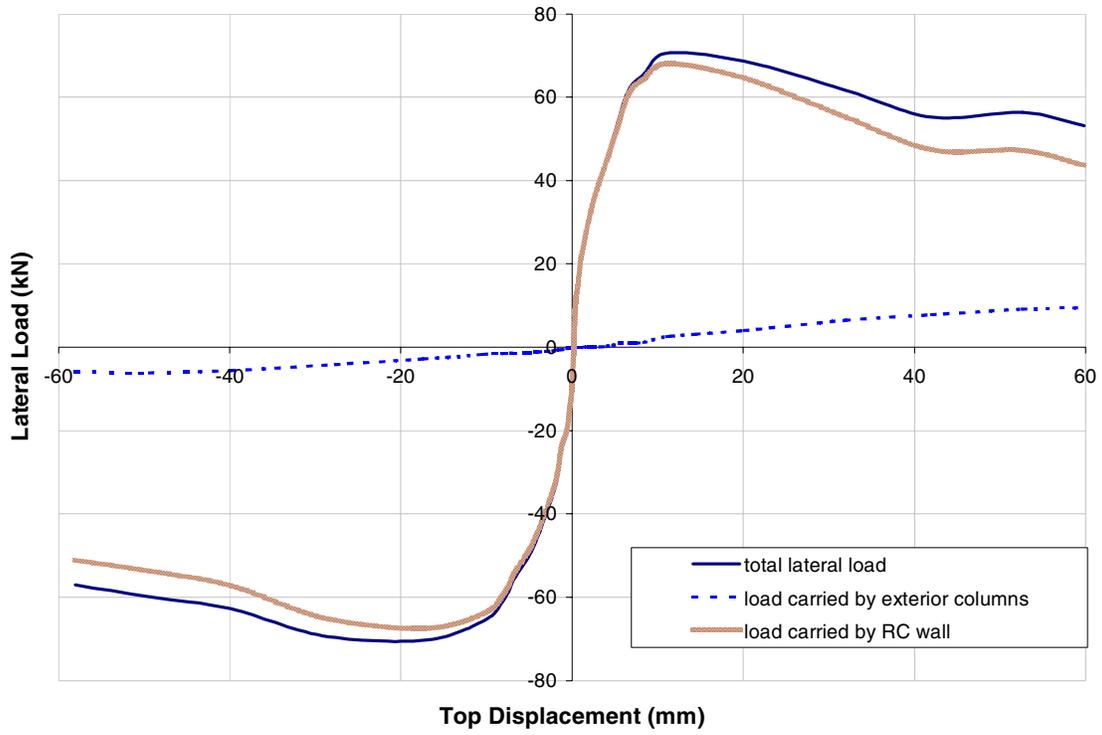
**Figure 9. Load Sharing Envelopes of the Members of Specimen S1**
