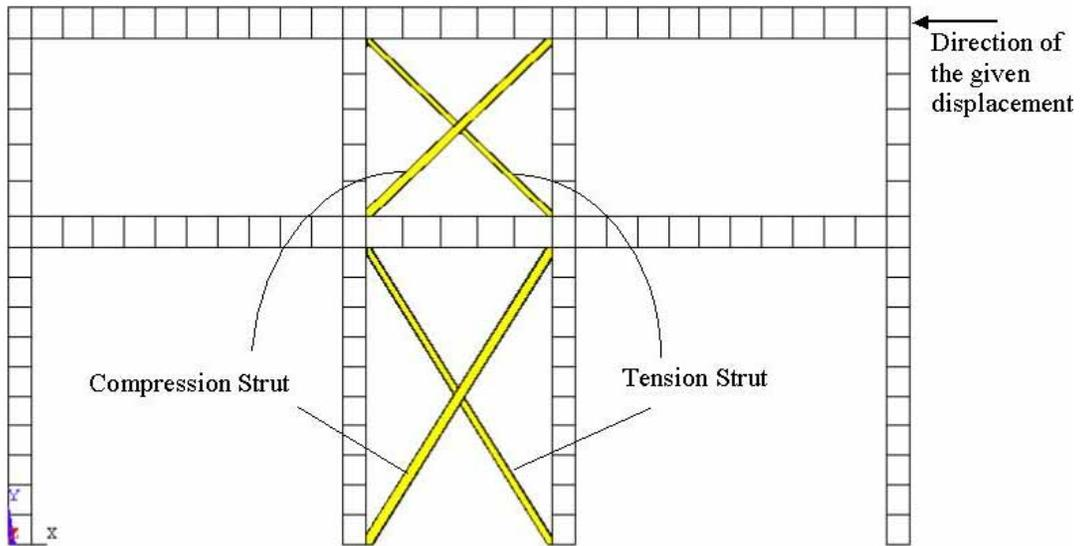
**Figure 12. Finite Element Model of Specimen S2**
