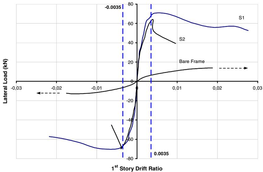
**Figure 8. First Story Drift Ratio Envelopes of the Specimens**
