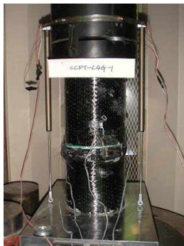
Fig.3. Axial compression test setup.
