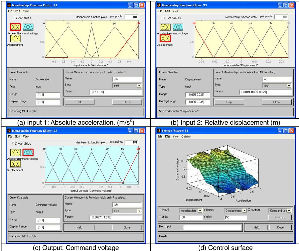
**Figure 3: Input and output membership functions of semi-active control surface “S3”.**
