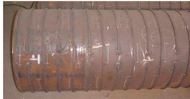
Photo.2 Shape of steel pipe with outer ribs
