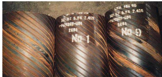
Photo.1 Steel pipe with outer ribs
