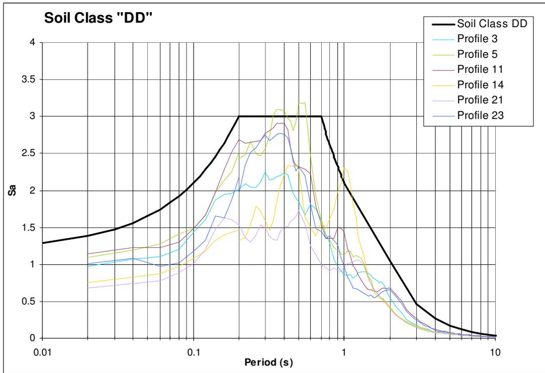
**Figure 14: Proposed Soil Class "DD"**
