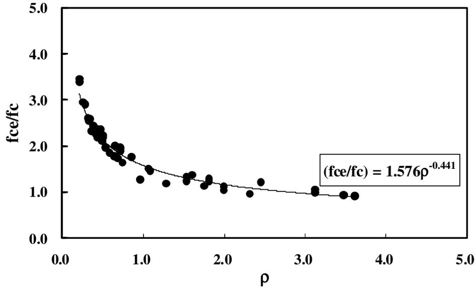
Fig. 9. Non-dimensional compressive load of confined concrete versus  $\rho$
