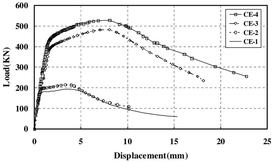
(a) Hollow section specimens
