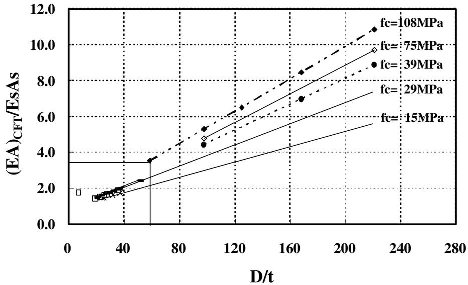
Fig. 7 Relationship between the ratio of axial stiffness and D/t
