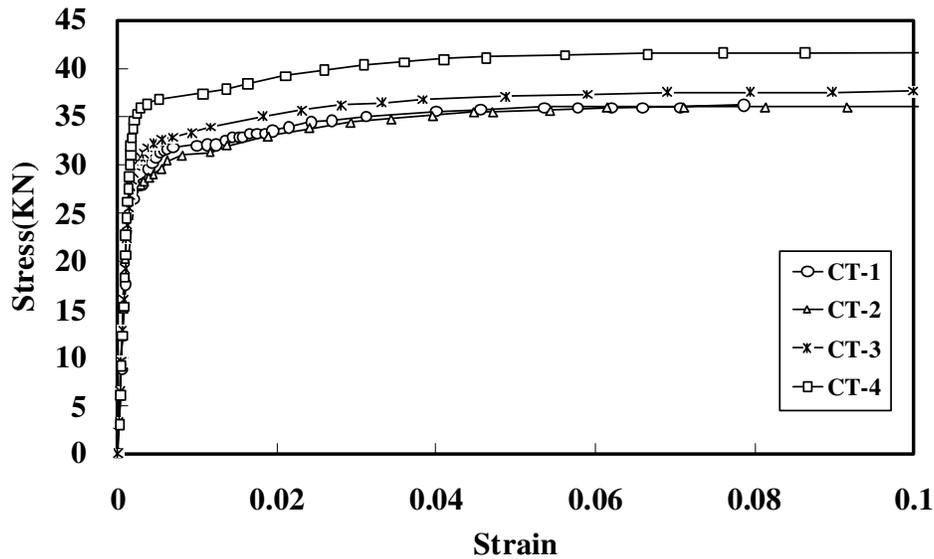
**Fig. 1. Stress-strain curves of steel coupon**
