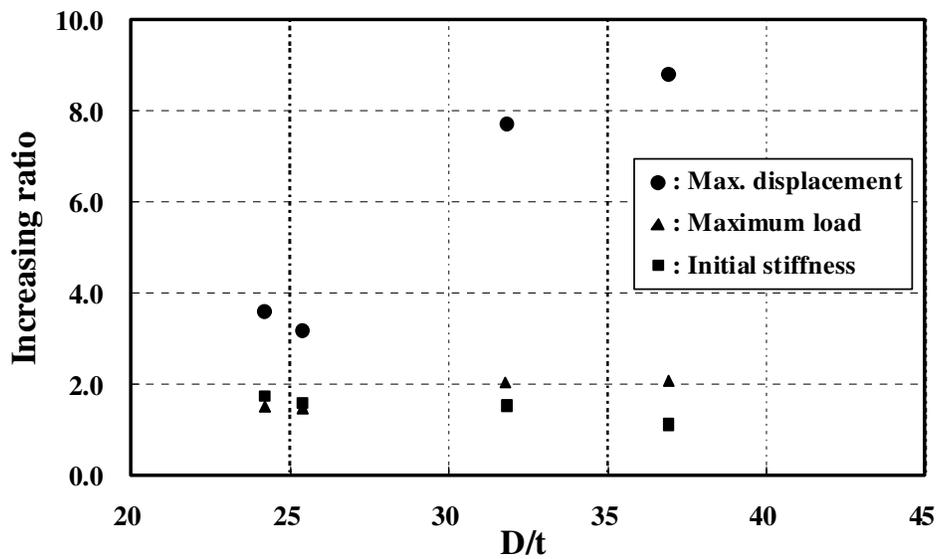
**Fig. 4. Comparison of increasing ratio due to filling the concrete and D/t**
