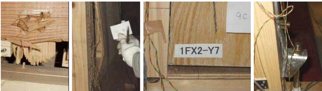
(a) Broken column      (b) Buckled plywood      (c) Gap of plywood and sill      (d) bend of Hold-down
