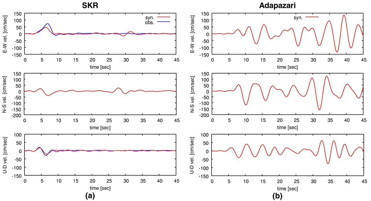
**Figure 9: Simulated waveform using 3D model and observed ones, (a) E-W, N-S, U-D waveforms at SKR, (b) E-W, N-S, U-D waveforms at downtown of Adapazari.**
