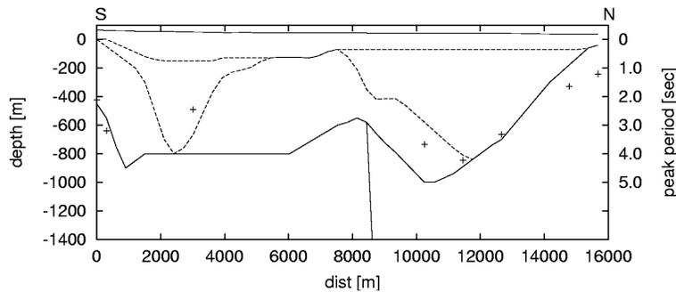
**Figure 3: Comparison between predominant periods (+) and depth of bedrock along the refraction/reflection survey line.**
