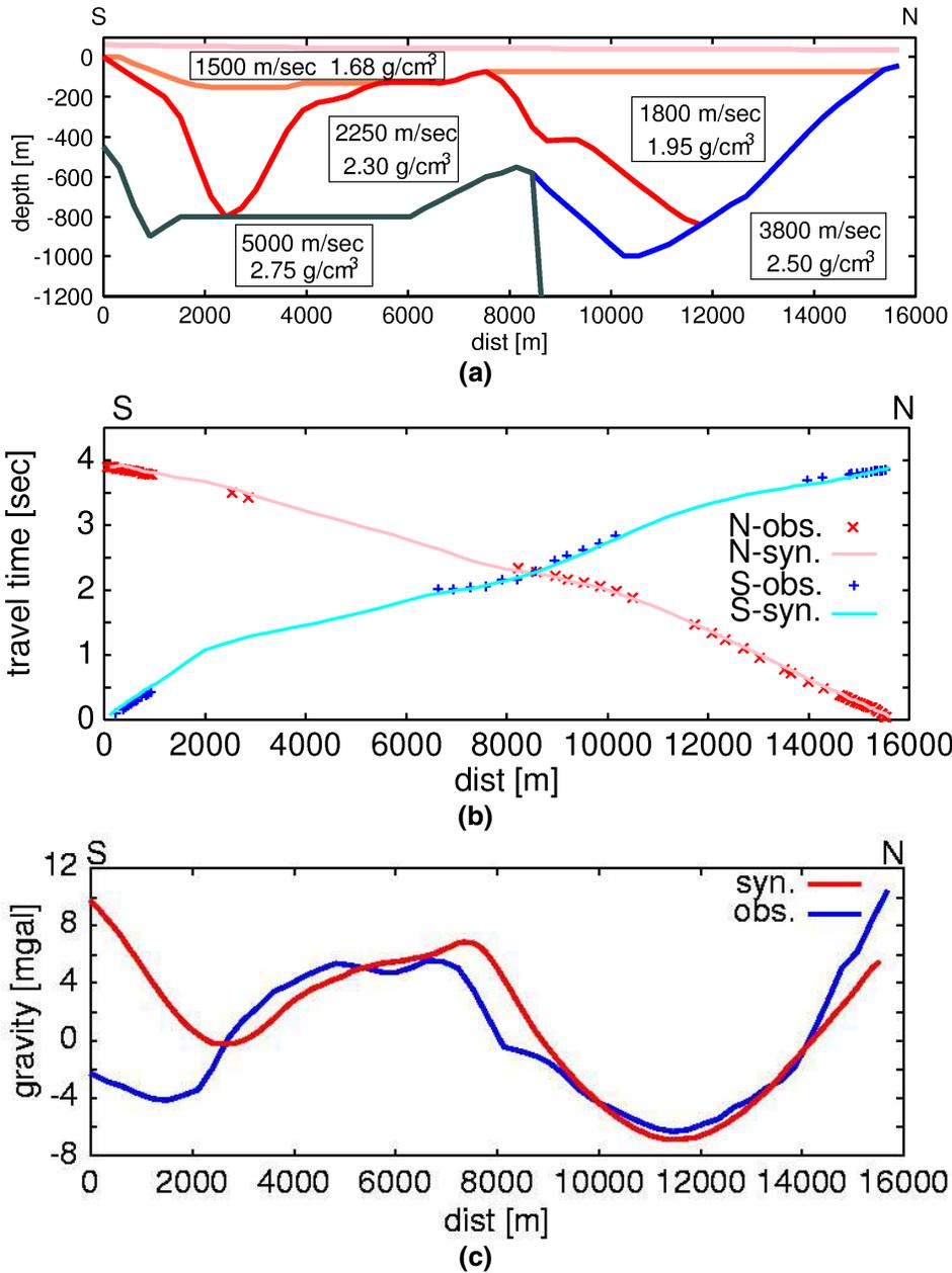
**Figure 2: The proposed 2D model under the survey line, Goto *et al.* [3], (a) proposed 2D model (P-wave velocity [m/sec] and density [g/cm<sup>3</sup>]), (b) calculated first travel times for both blasts, (c) observed gravity anomaly except a trend component and calculated one.**
