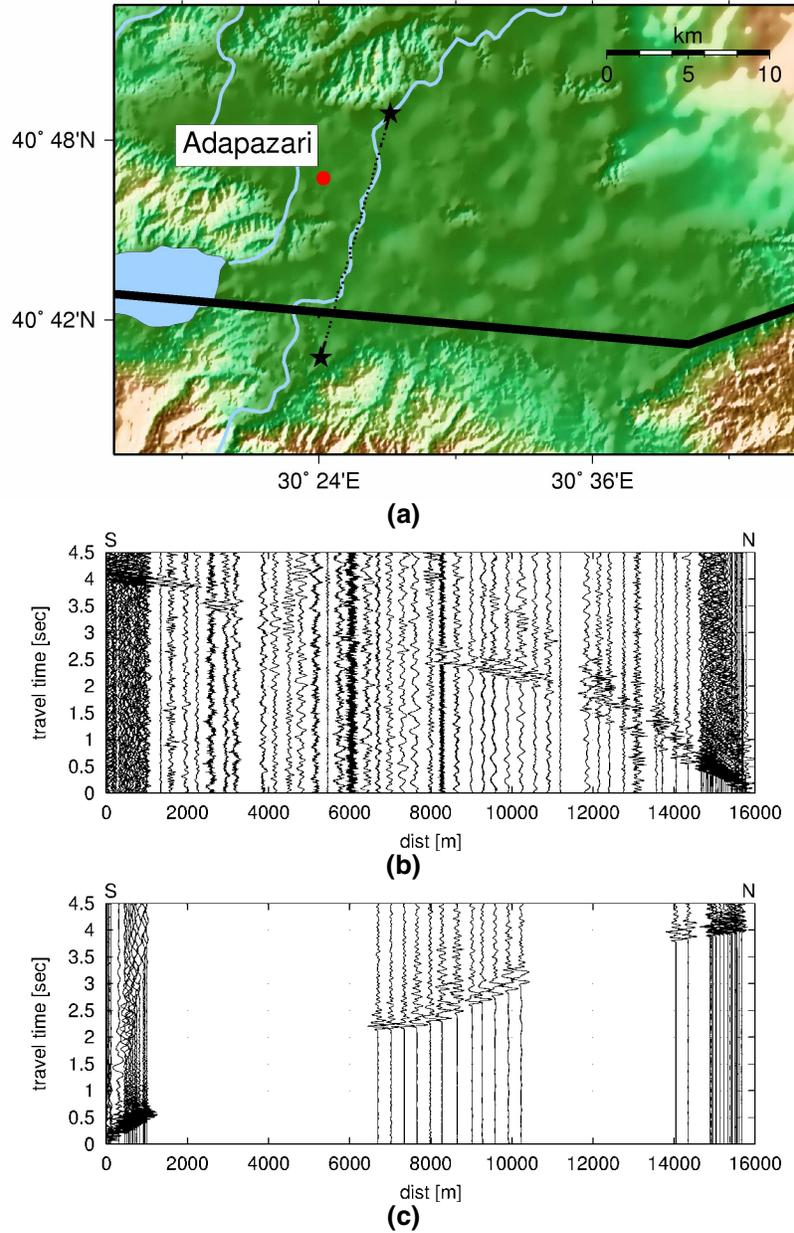
**Figure 1: The seismic refraction and reflection survey, (a) location of blasts (★) and receivers (•), (b) the records for the northern blast, (c) the records for southern blast.**
