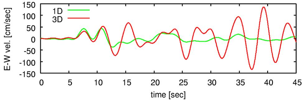
**Figure 10: Comparison between simulated waveform (E-W) by 3D and 1D model.**
