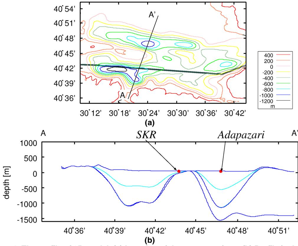
**Figure 4: The profile of 3D model, (a) Location of the cross sections, (b) Profile included Adapazari and SKR (A-A').**
