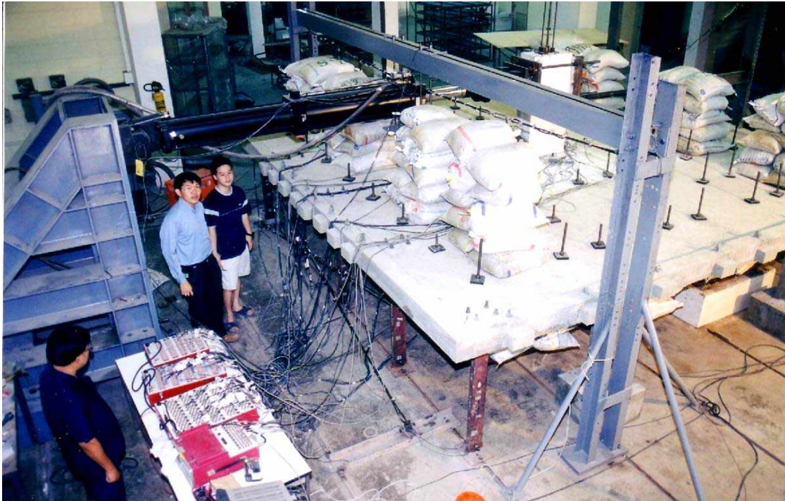
Figure 9: A cyclic loading test of a 3/5 scaled interior post-tensioned flat slab-column connection
