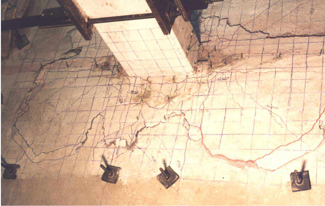
Figure 10: Punching shear failure at the slab-column connection
