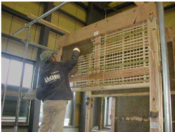
Photo 1: Plastering the test specimen.
