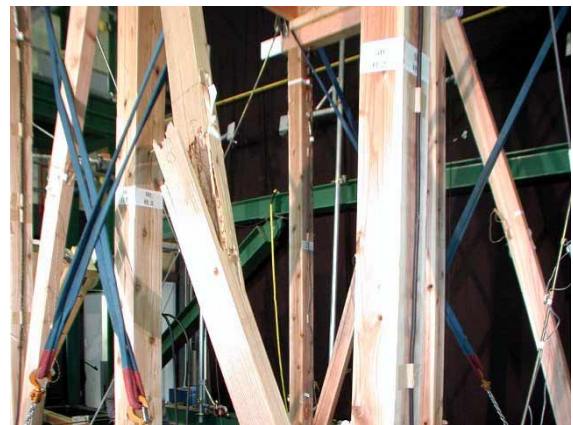
Photo 6 : [Wooden-brace test] Broken wooden brace.
