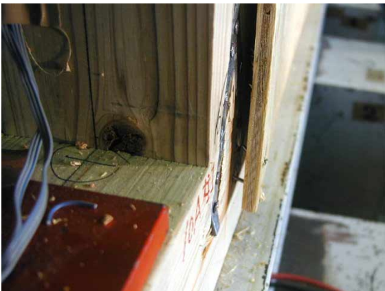
Photo 7 : [Plywood-wall test] Out-of-plane buckling of a plywood panel.
