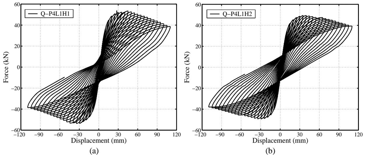
**Figure 6 Q-type columns with short lapping and 4 FRP layers applied over: (a) 0.3m; (b) 0.6m.**
