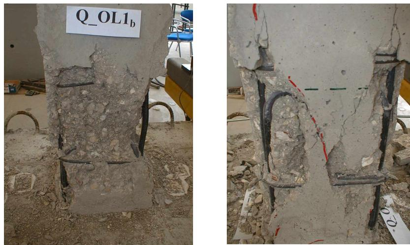
**Figure 4 Failure of non-retrofitted type-Q specimens:
