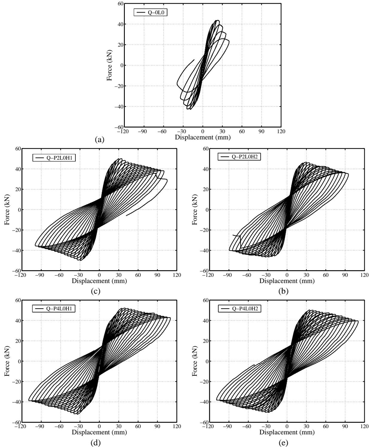
**Figure 3 Q-type columns without lap splices: (a) Q-0L0, un-retrofitted; (b) Q-P2L0H1, 2 CFRP layers over 0.6m; (c) Q-P2L0H2, 2 CFRP layers over 0.3m; (d) Q-P4L0H1, 4 CFRP layers over 0.3m; (e) Q-P4L0H2 4 CFRP layers over 0.6m**
