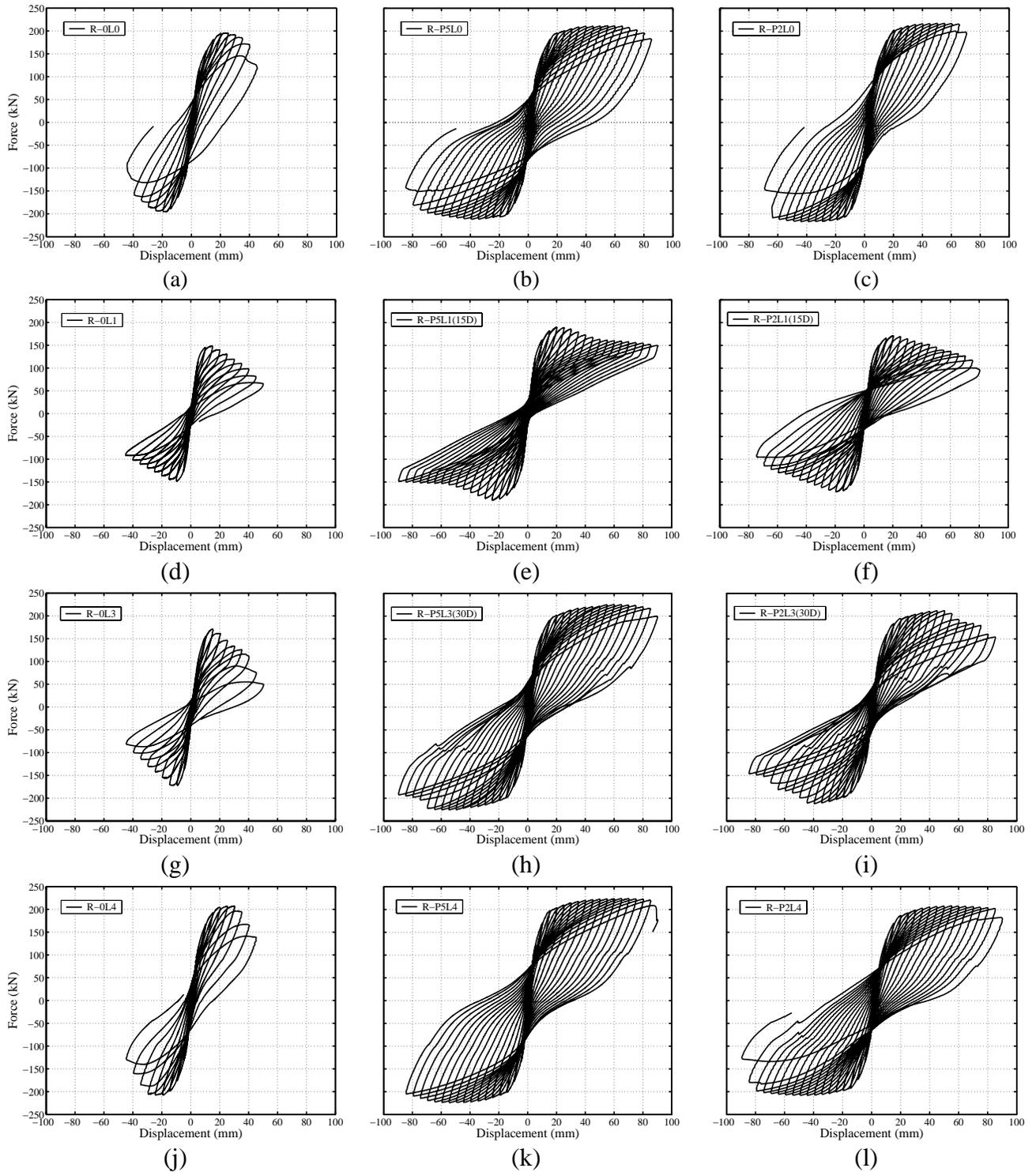
**Figure 7** Effect of lap-splice length in R-type columns, un-retrofitted (left): (a) R-0L0, (d) R-0L1, (g) R-0L3, (j) R-0L4; retrofitted with 5 CFRP layers, (center): (b) R-P5L0, (e) R-P5L1, (h) R-P5L3, (k) R-P5L4; retrofitted with 2 CFRP layers (right): (c) R-P2L0, (f) R-P2L1, (i) R-P2L3, (l) R-P2L4
