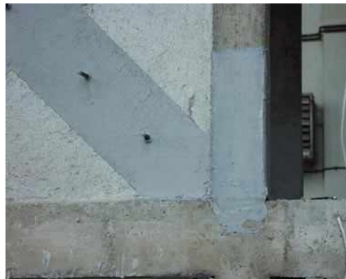
Fig. 8 Specimen 2: Completed model with added carbon fibers
