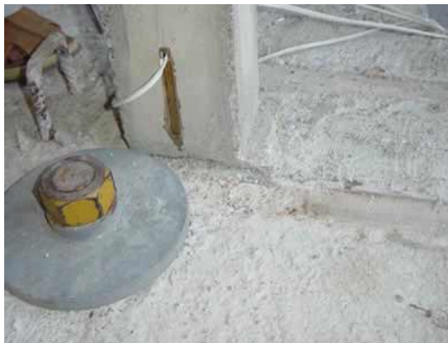
Fig. 13 Specimen 1: Brittle shear-slip failure between the columns and foundation due to inadequate stirrup lap-splice-length
