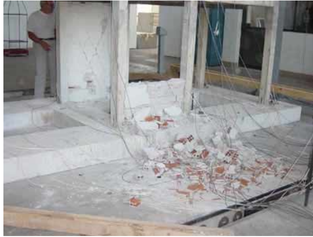
Fig. 12 Specimen 1: Shear-slip failure between the concrete elements and masonry infill wall due to poor connection
