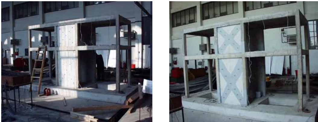
Fig. 7 Specimen 2: step 1(left) - anchorage holes are drilled; step 2(right) –anchor dowels are put
