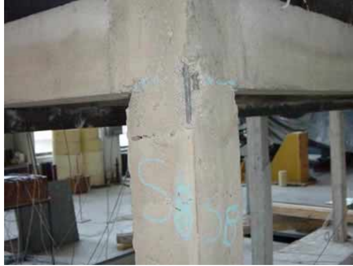
Fig. 14 Specimen 1: Crushing and spalling of concrete
