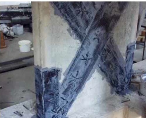
Fig. 9 Specimen 2: Some details of CFRP incorporation
