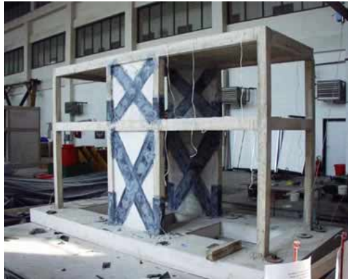
Fig. 8 Specimen 2: Completed model with added carbon fibers
