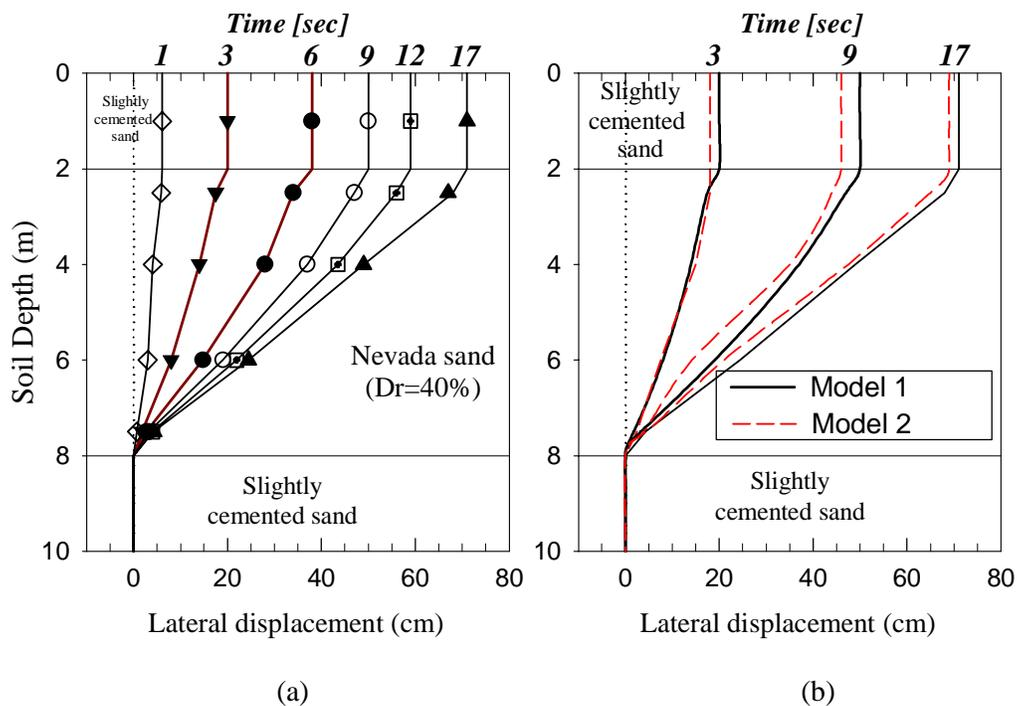
**Figure 4. Free-field lateral displacement profiles at different times during shaking (a) in Model 1; (b) comparison of Models 1 and 2.**
