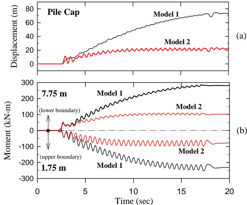
**Figure 5. (a) Comparison of pile head lateral displacements in Models 1 and 2; (b) bending moment time histories measured in downslope piles in Model 2.**
