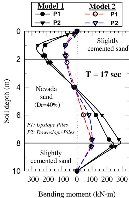
**Figure 6. Comparison of measured bending profiles in upslope and downslope piles at the end of shaking for Models 1 and 2.**
