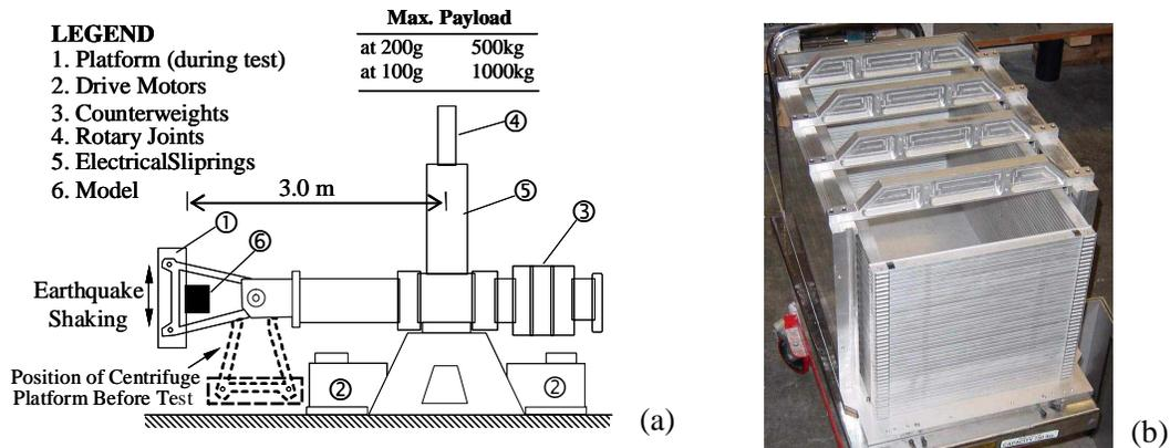
**Figure 1. (a) Sketch of RPI's dynamic geotechnical centrifuge, (b) large laminar box.**
