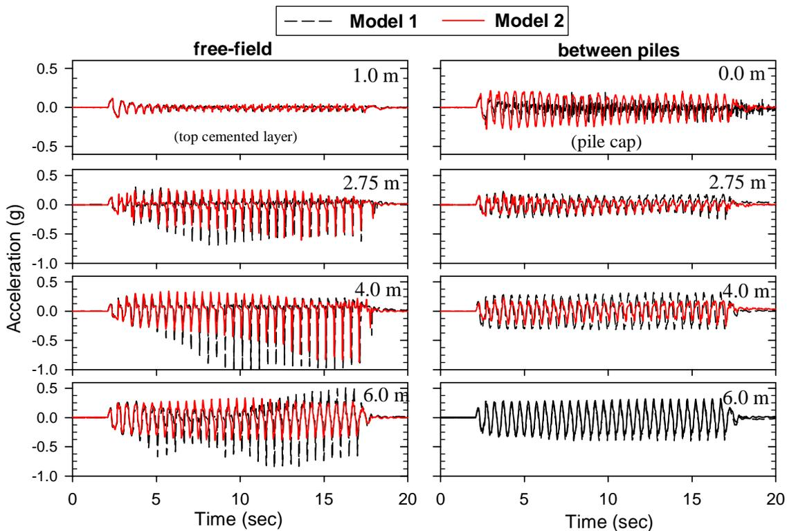
**Figure 3. Comparison of accelerations measured in the horizontal direction in free-field and pile group core, and on the pile cap, Models 1 and 2.**
