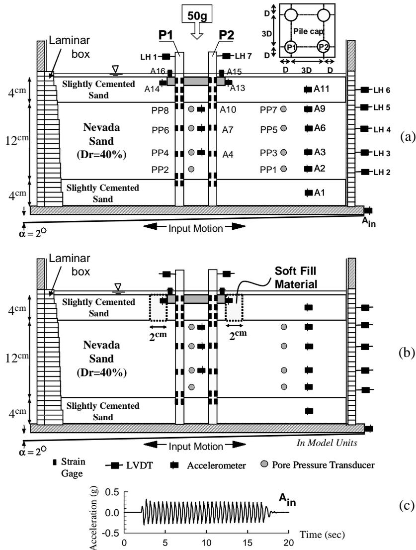
**Figure 2. Setups and instrument locations of centrifuge models: (a) Model 1; (b) Model 2, and (c) prototype base acceleration.**
