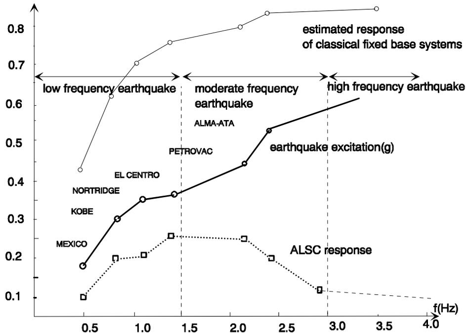
Fig.4 Performance of the model isolated by ALSC system under earthquake excitation
