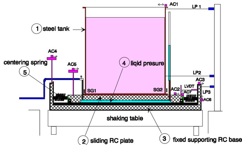
Fig.2. Instrumentation set-up
