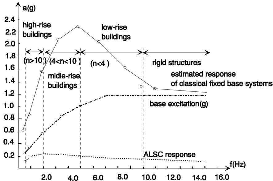
Fig. 3 Performance of the model isolated by ALSC system under harmonic excitation
