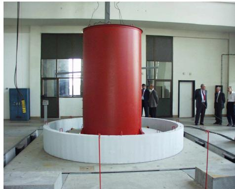
**Figure 1. "ALSC" system applied on steel liquid storage tank model**
