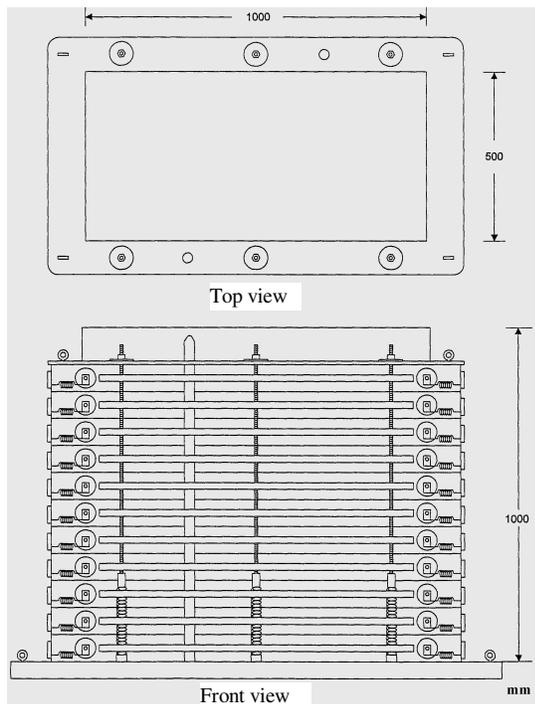
**Fig.1. Layout of Laminar box**
