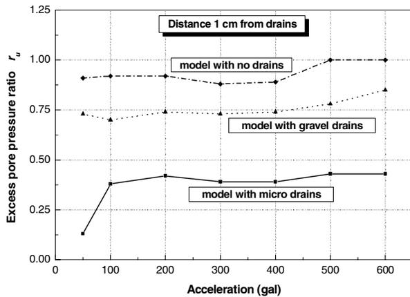
**Fig.9. Max  $r_u$  at 1 cm from drains**
