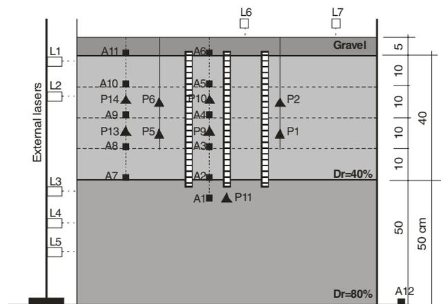
■ Accelerometer (A) □ Laser transducers (L)
