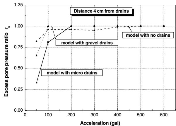
**Fig.10. Max  $r_u$  at 4 cm from drains**
