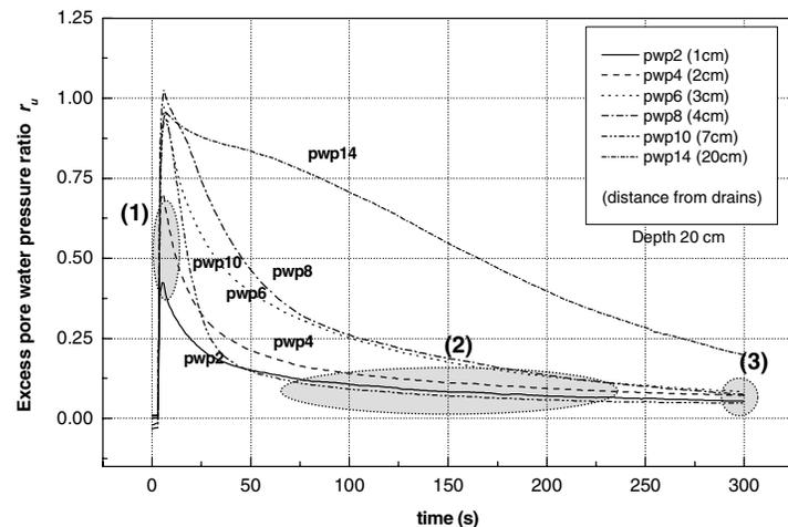
Fig.8. Dissipation of  $r_u$  – ADRA model
