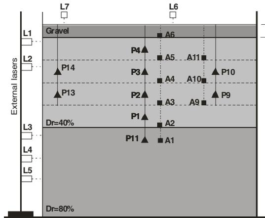
■ Accelerometer (A) □ Laser transducers (L)
