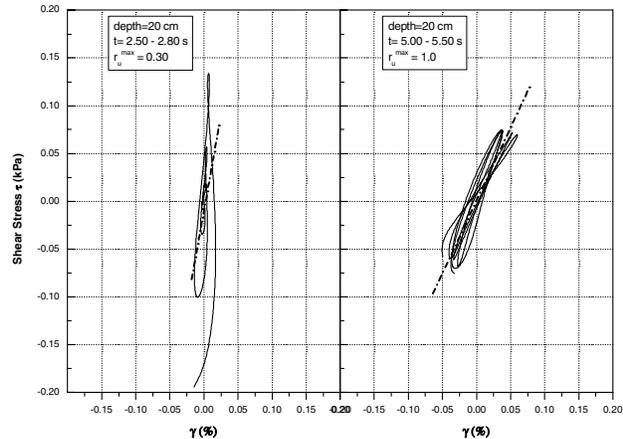
Fig.6. Shear stress-strain relationship - BDRA
