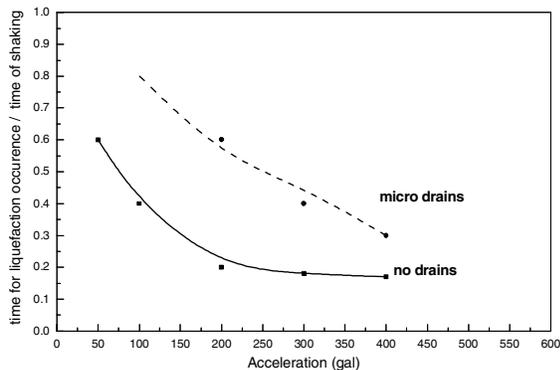
**Fig.11. Necessary time for liquefaction**
