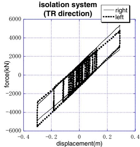
**Figure 10. Hysteresis Loops of Sliding Bearings and Isolation Systems**
