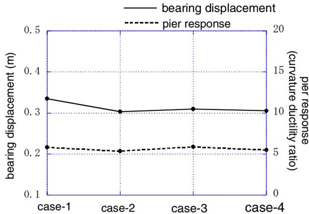
**Figure 7. Result of Analysis paying Attention to Velocity and Bearing Pressure Dependence of the Friction coefficient**
