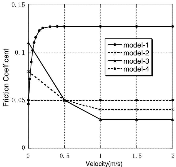
**Figure 5. Velocity Dependence of Friction Coefficient**
