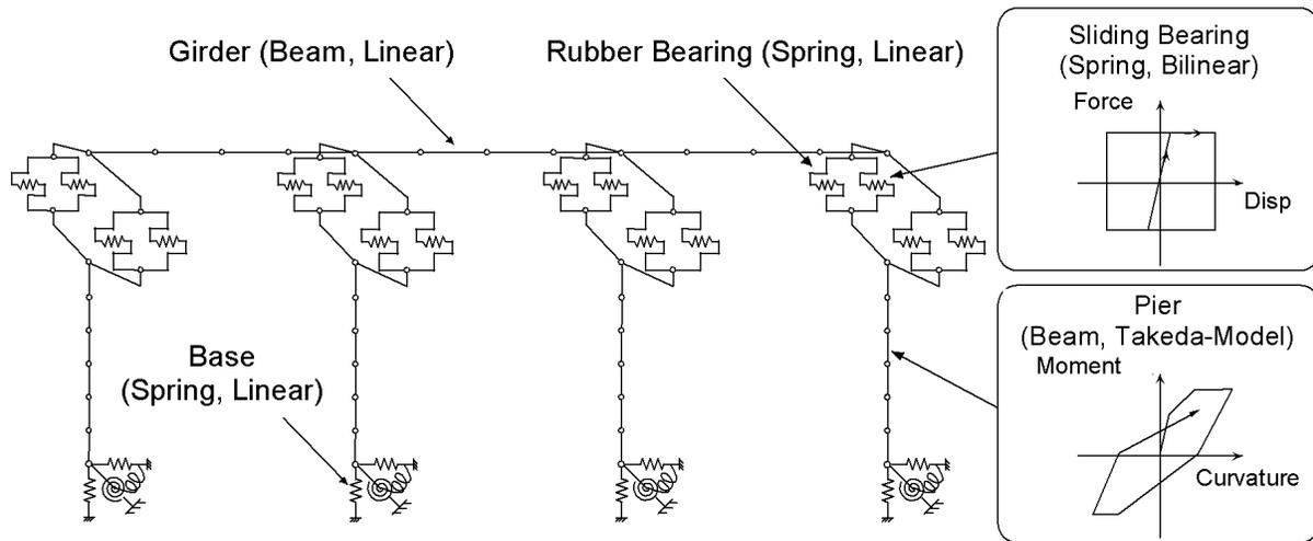
Figure 2. Model of the Bridge
