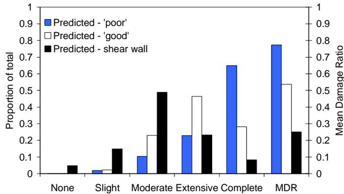
**Figure 10: Sensitivity of damage estimations to building vulnerability model for mid-rise RC frame buildings using best estimate ground shaking demand (no liquefaction).**
