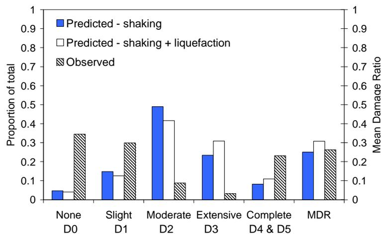
**Figure 7: Predicted vs. observed damage to mid-rise RC frame buildings in central Adapazari.**
