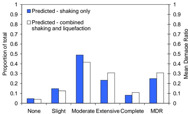
**Figure 11: Sensitivity of damage estimations to the incorporation of liquefaction induced damage for mid-rise RC frame buildings with infill walls.**
