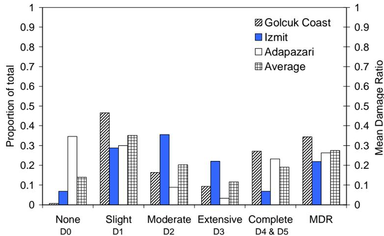
**Figure 6: Comparison of Adapazari structural damage to Gölcük coastal zone and Izmit survey area. Mean damage ratio, MDR assumes 2% loss for slight damage, 10% for moderate damage, 50% for extensive damage and 100% loss for complete damage (Bommer et al. [7]).**
