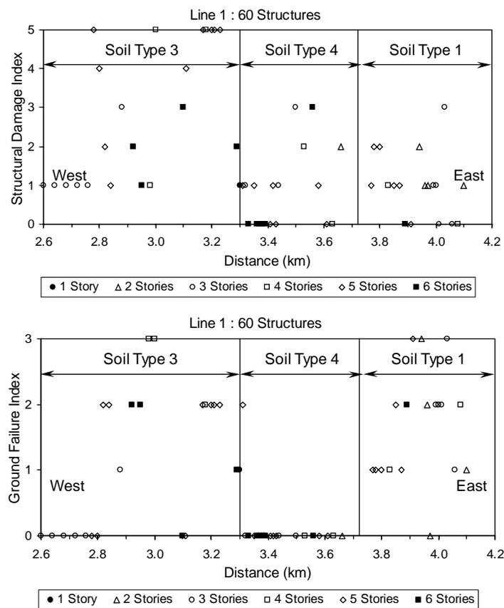
**Figure 8: Correlations between structural damage index (Table 1) and ground failure index (Table 2) for a portion of line 1 of Bray & Stewart’s [2] survey data (Figure 2).**
