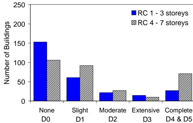
**Figure 5: Distribution of building damage to RC frame buildings in central Adapazari survey zone. See Table 1 for definitions of damage states**
