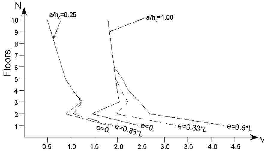
**Figure 4: Variation of coefficient  $v$  versus the increase of number of stories and of the ratio  $a/h_c$ .**
