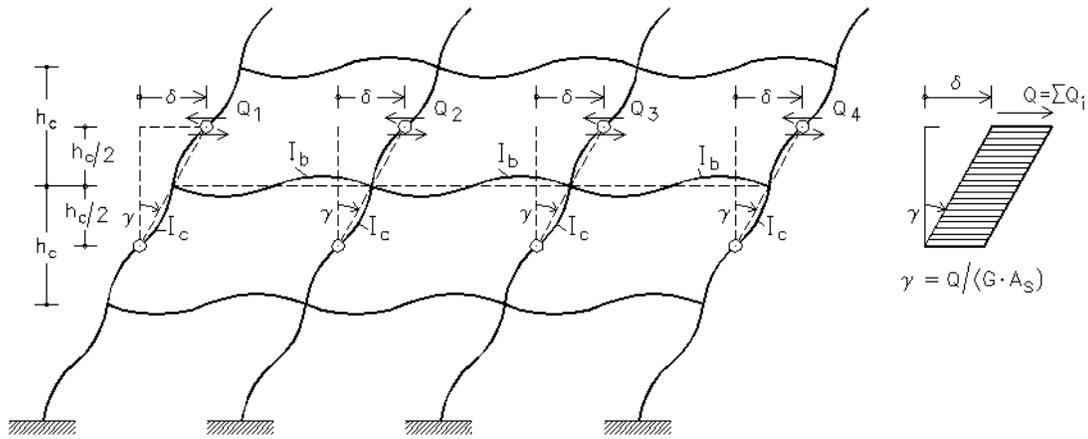
**Figure 1. Formation of the continuous model of the shear subsystem**
