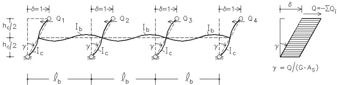
**Figure 2. Determination of the equivalent shear stiffness of the frame**
