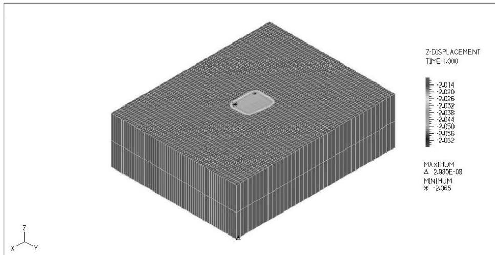
**Figure 5: Settlements under the foundation**
