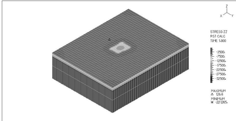
**Figure 4: Pressure under the foundation**
