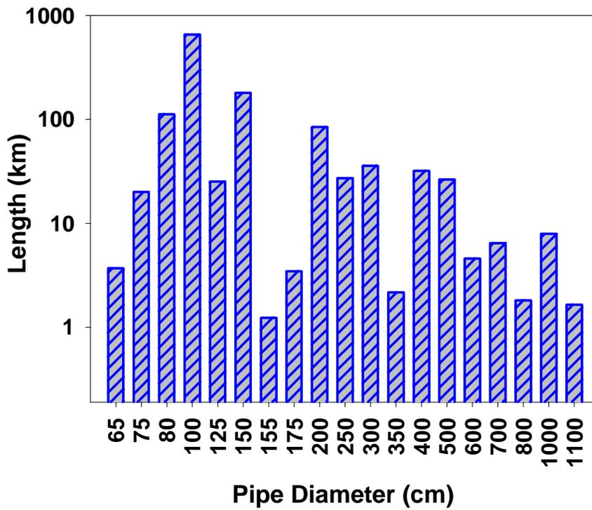
(a) Length of Pipelines with respect to Pipe Diameter
