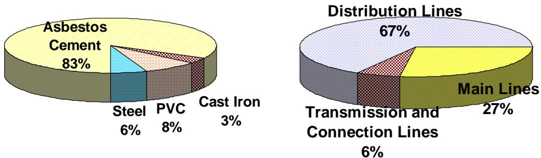
(b) Relative Lengths of Pipelines with respect to Pipe Composition
