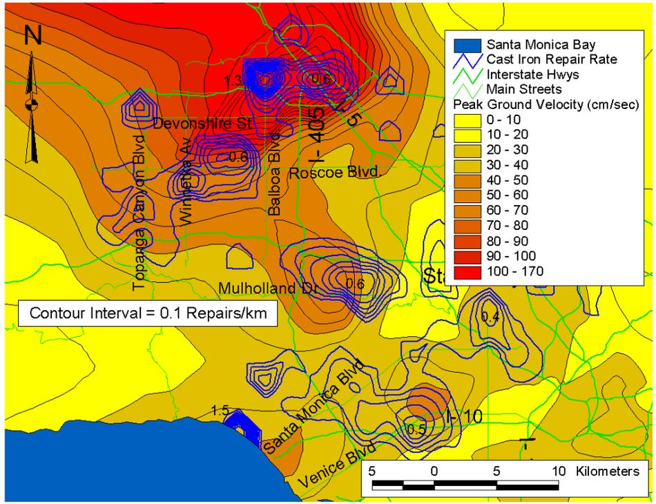
**Figure 5. Pipeline Repair Rate Contours Relative to Northridge Earthquake Peak Ground Velocity O'Rourke [10]**
