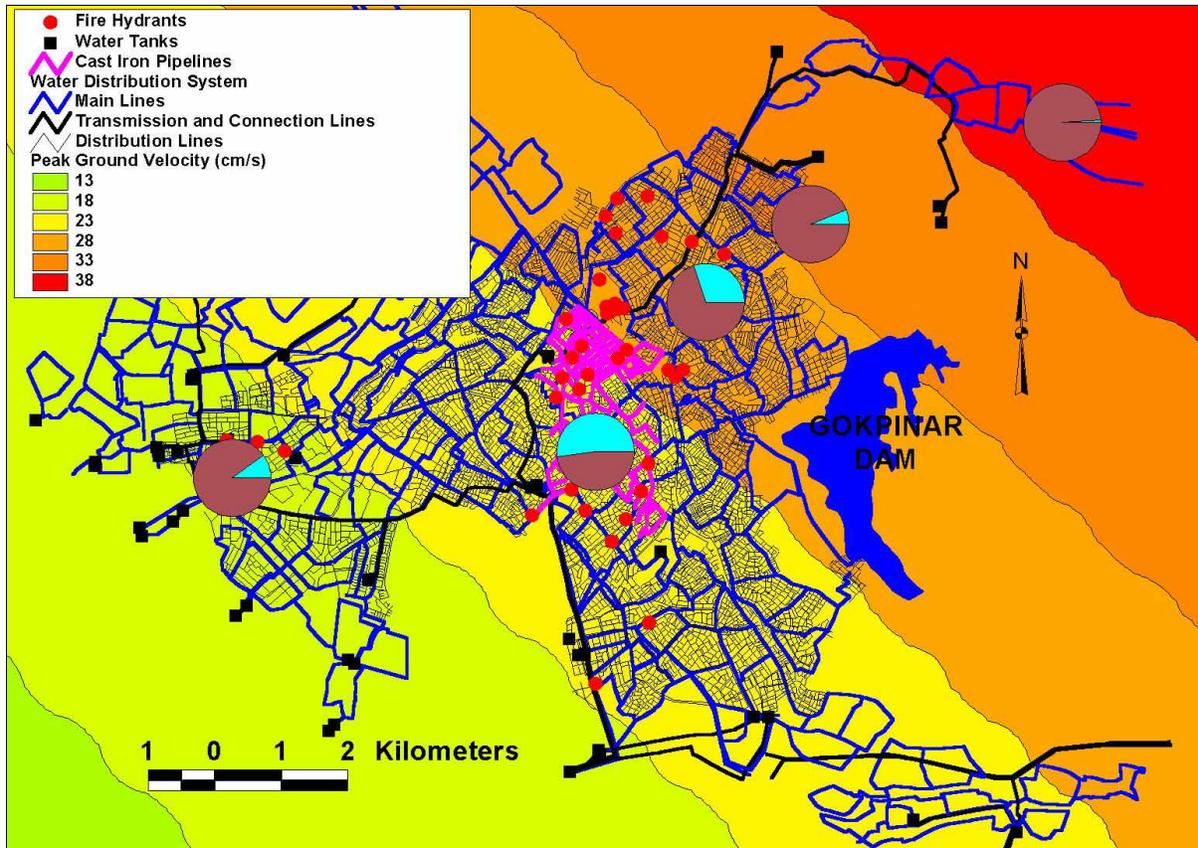
Figure 7. Water Supply System Relative to Denizli Scenario Earthquake Peak Ground Velocity
