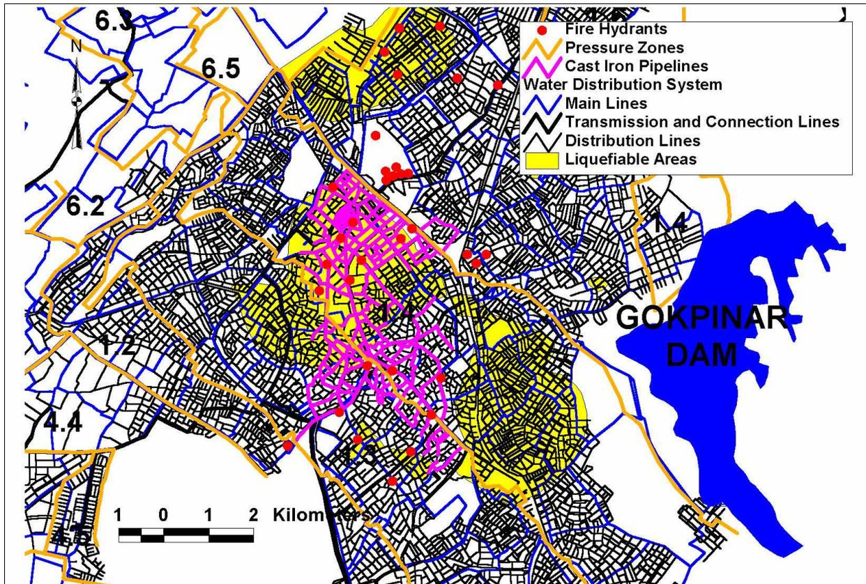
**Figure 8. Water Supply System Relative to Liquefiable Areas**
