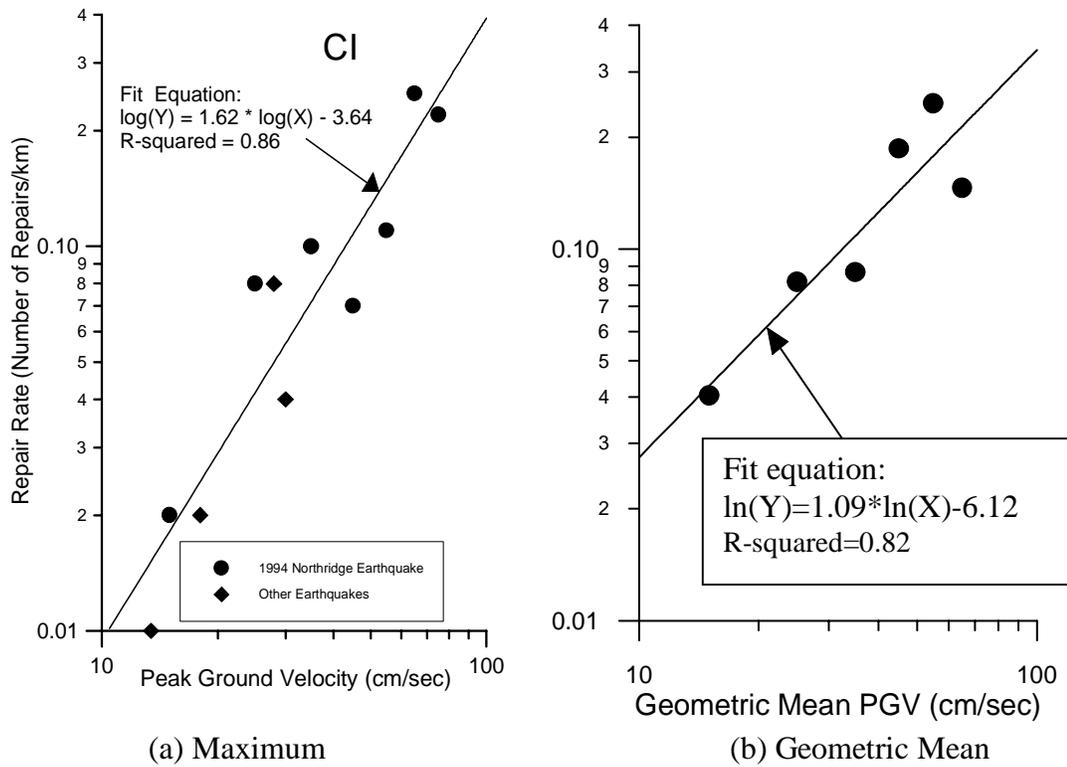
**Figure 6. CI Repair Rate Regression with Maximum Toprak [9] and Geometric Mean of PGV O'Rourke [14]**
