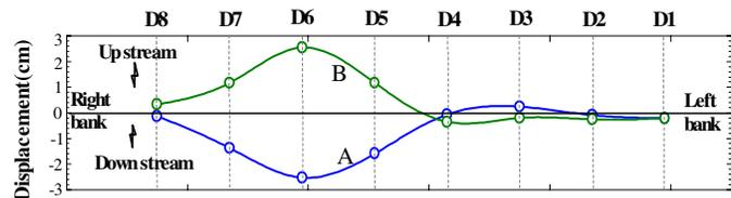
Fig.16 Displacement mode on dam crest at time A and B
