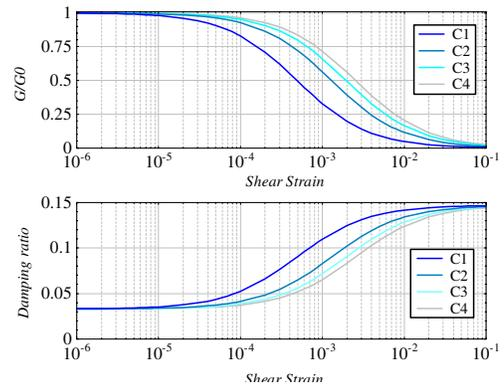
Fig.10 Strain dependence curve
