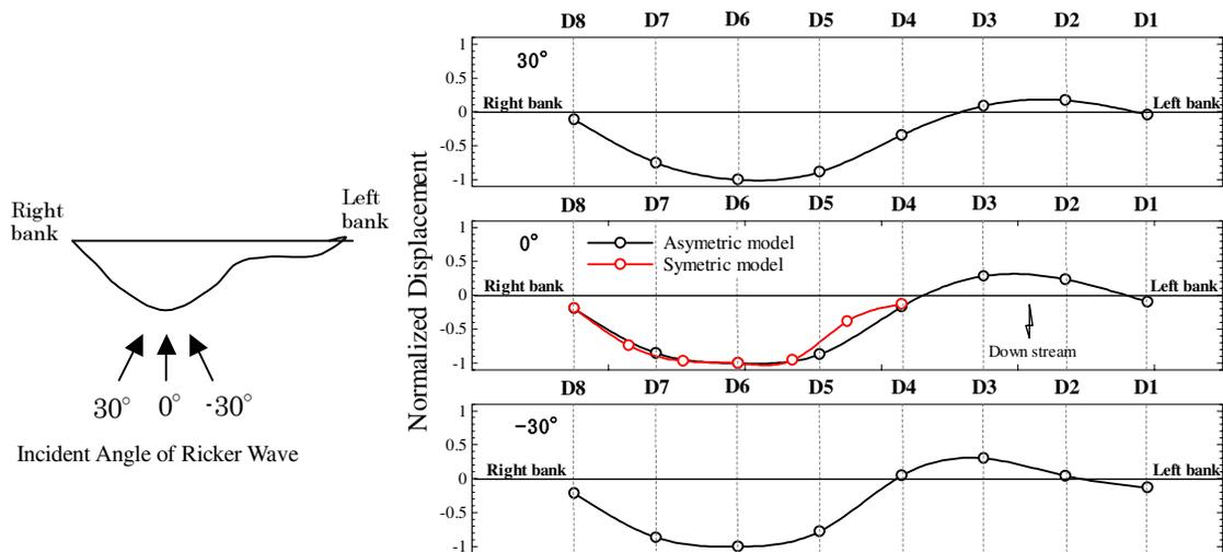
Fig.17 Behavior of the displacement on dam crest in each incidence angle
