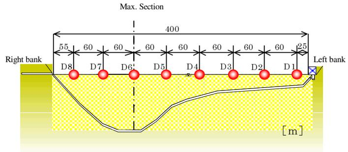
Fig.14 Output point of dam crest
