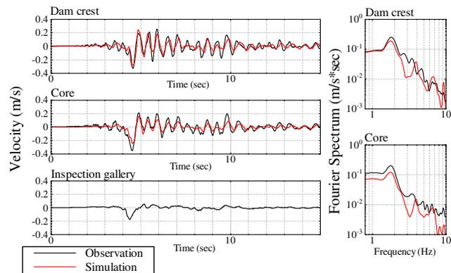
Fig.13 Comparison of analysis with observation for up-down stream direction of dam axis model
