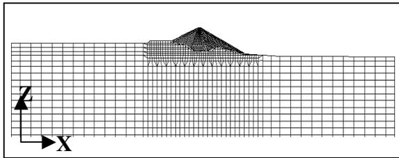
Fig.6 Section model of up-down stream direction
