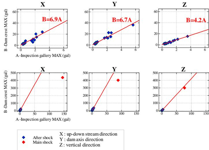
Fig.3 Distribution of maximum acceleration amplification factor
