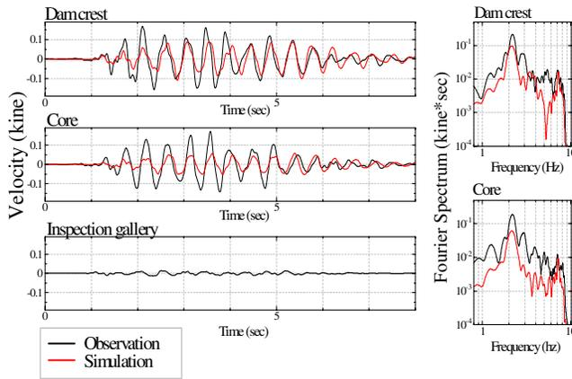
Fig.8 Comparison of analysis with observation for up-down stream direction
