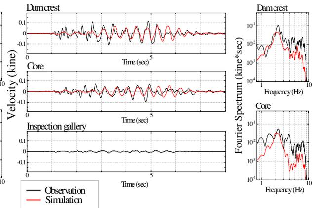
Fig.9 Comparison of analysis with observation for dam axis direction
