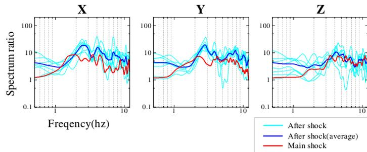
Fig.4 Transfer function between dam bottom and crest
