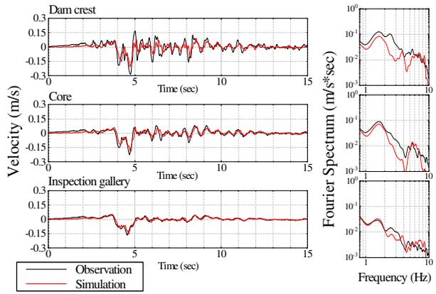
Fig.12 Comparison of analysis with observation for dam axis direction
