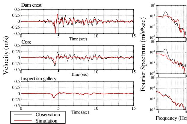
Fig.11 Comparison of analysis with observation for up-down stream direction
