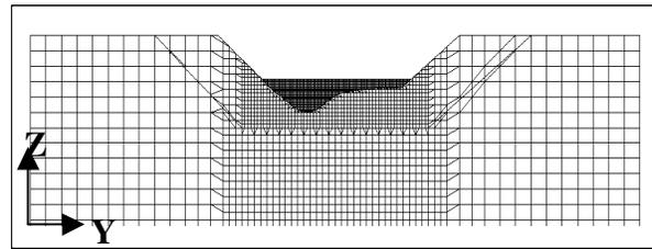
Fig.7 Section model of dam axis direction
