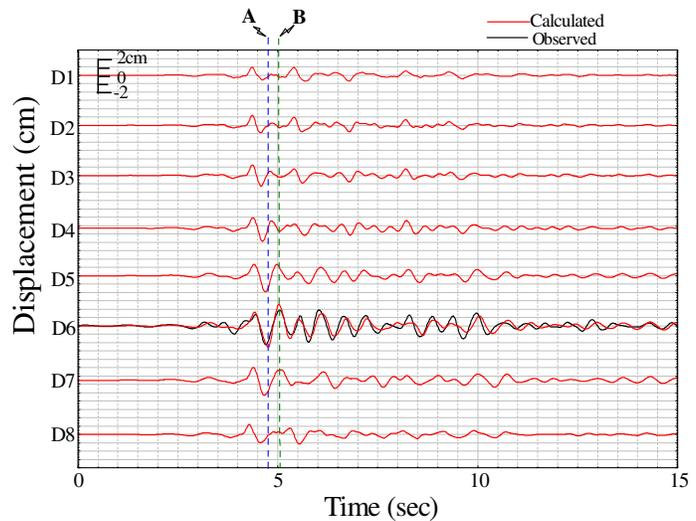
Fig.15 Displacement behavior on dam crest
