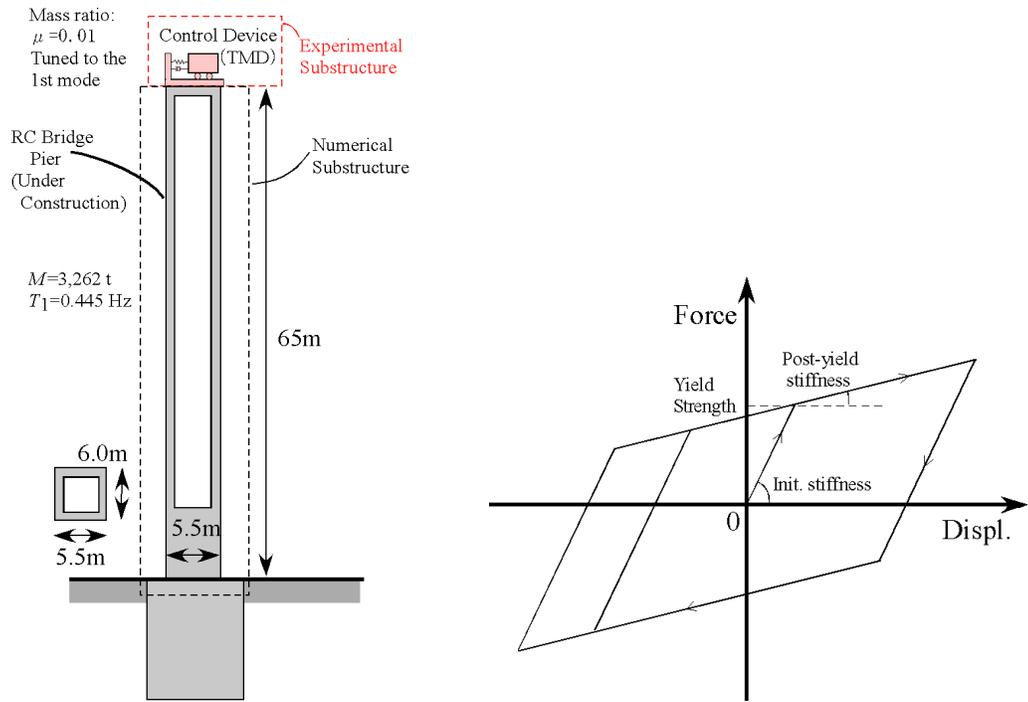
(a) Model structure: Pier-TMD system      (b) Bilinear model for the nonlinearity of the Pier
