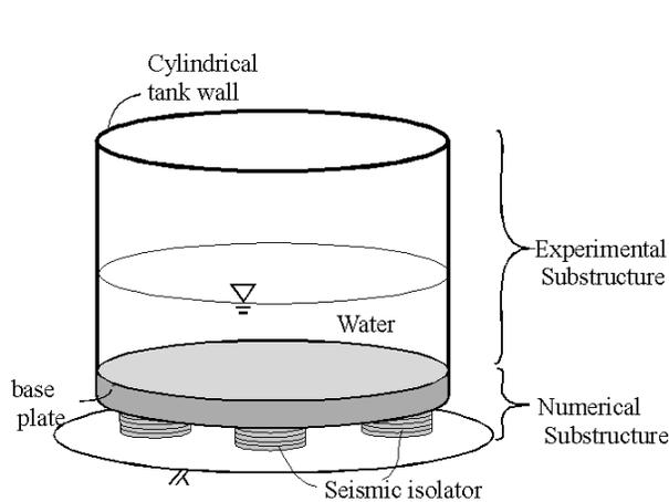
Fig. 11 Concept of the application to the seismically isolated liquid storage tanks
