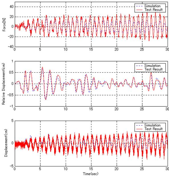
Fig. 15 Test result:  $P_y = 0$  (elastic isolator)
