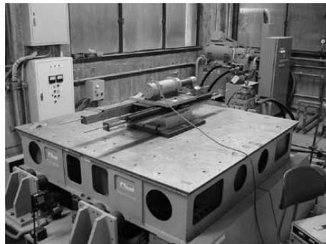
Fig. 2 Shake table for SHST test system development
