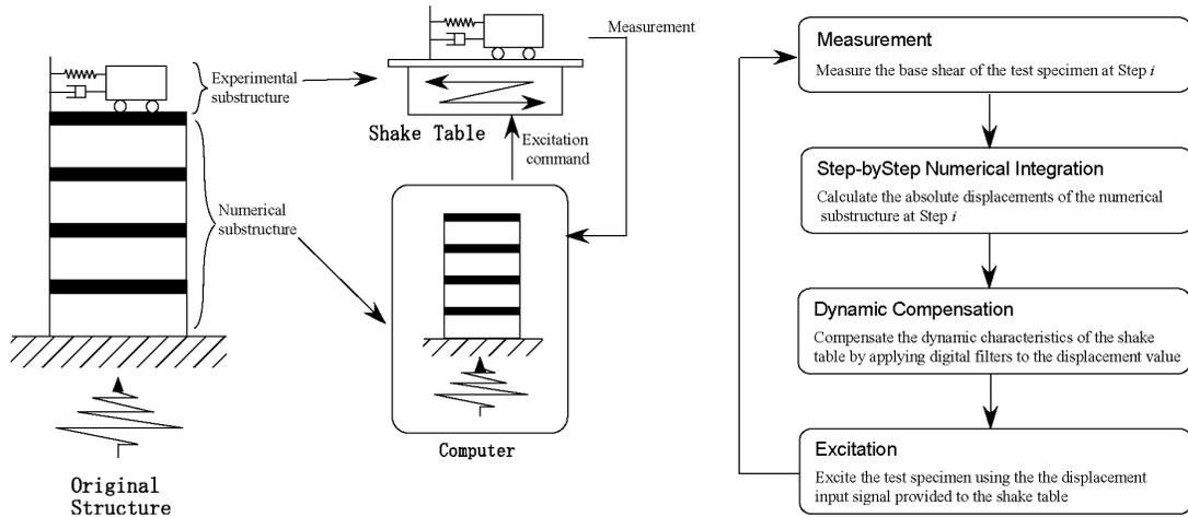
(a) Schematic of the test concept
