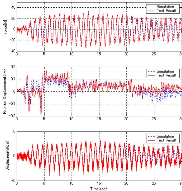
Fig. 17 Test result:  $P_y=0.02W$
