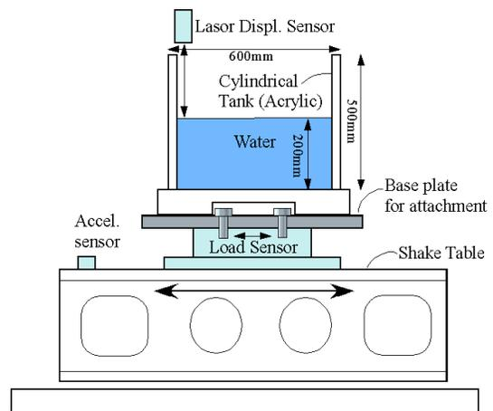
Fig. 12 Test setup for the liquid storage tank SHST tests
