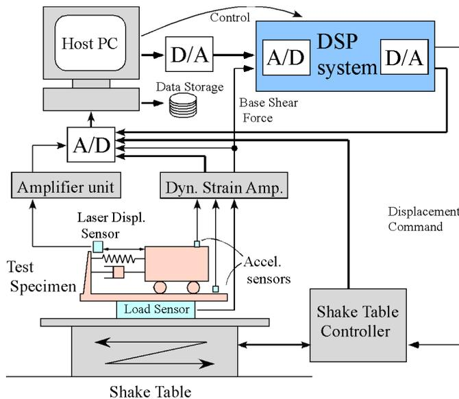
Fig.3 SHST Test System
