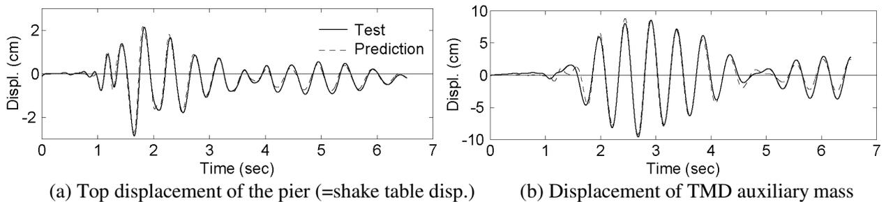
Fig. 9 Test result: Kobe JMA NS input (scale factor=1.3)
