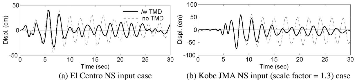
Fig. 10 Reduction of top displacement response of the pier (full-scale representation)
