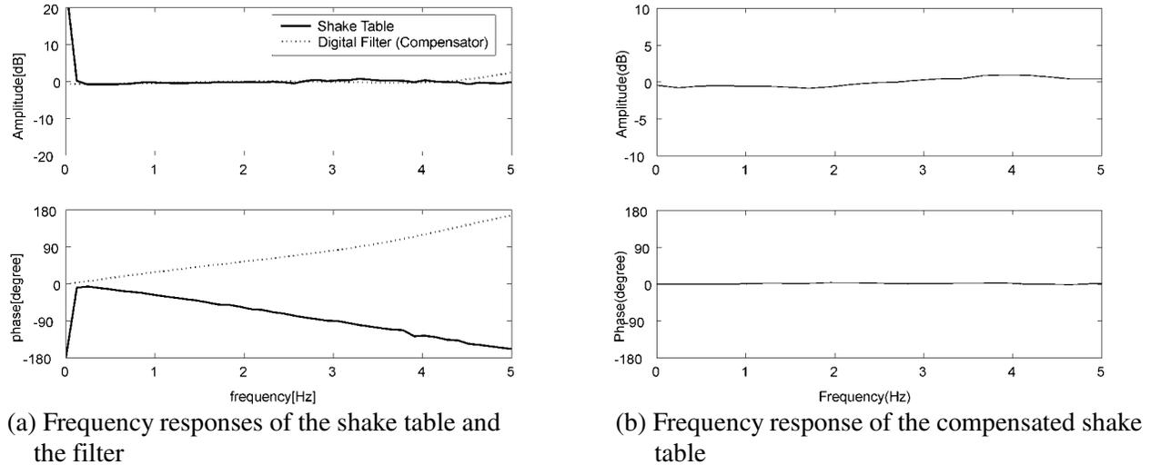
Fig. 4 Effects of dynamic compensation with respect to the frequency response
