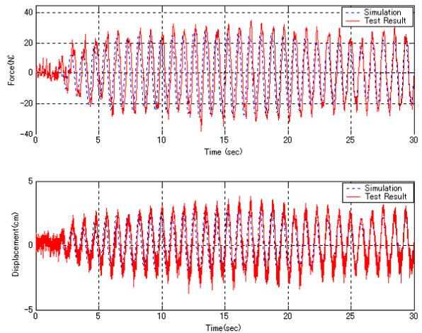
Fig.18 Response of the tank without seismic isolation
