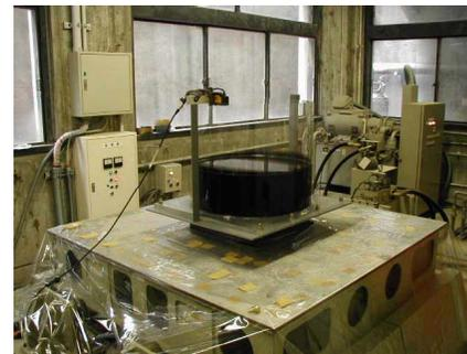
Fig.13 Liquid storage tank model on the shake table
