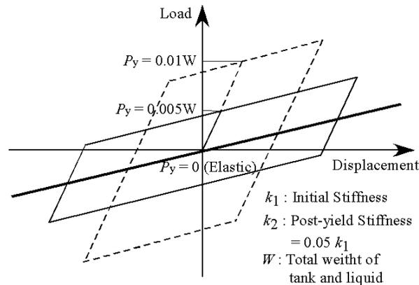
Fig. 14 Bilinear restoring force model for the seismic isolators
