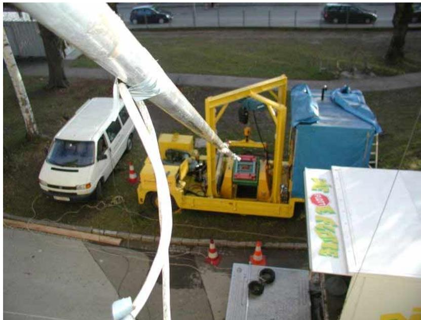
**Figure 1.1.:** reaction mass exciter, VICTORIA with rod-chain
