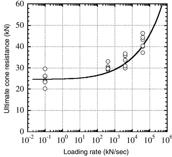
**Fig.5 Relationship between ultimate cone resistance and loading rate.**
