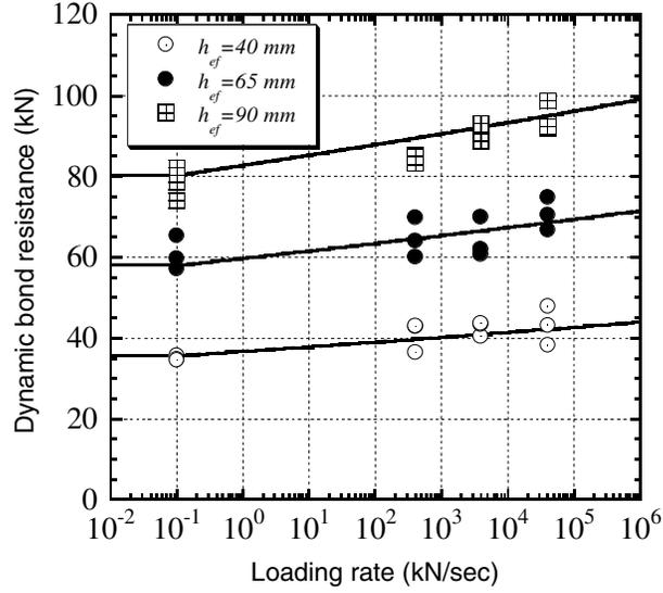
**Fig.6 Relationship between dynamic bond resistance and loading rate.**
