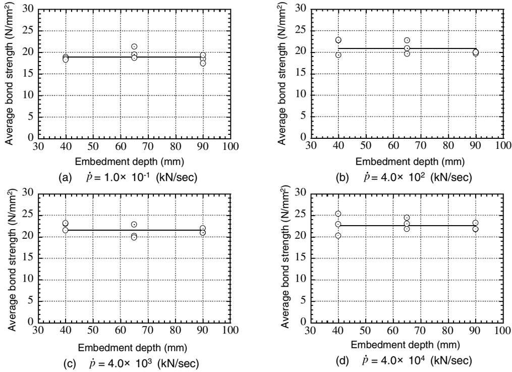
**Fig.7 Average bond strength and embedment depth.**
