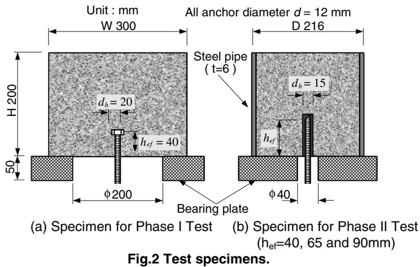
ultimate cone resistance (Phase I Test); 2) Rapid pullout loading tests of adhesive anchors, to examine the dynamic ultimate bond resistance (Phase II Test).
