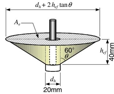
**Fig.4 Cone failure mode.**
