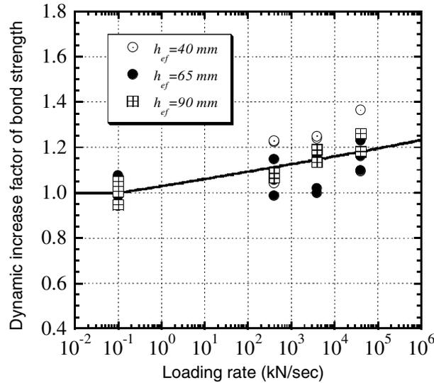
**Fig.8 Relationship between dynamic increase factor of bond strength and loading rate.**
