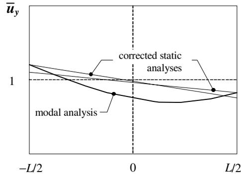
Figure 2. Application of corrected static analyses to a one-storey asymmetric system ( $\Omega_\theta=1.0$ ;  $T_y=1$  s;  $e_s=0.10 L$ )
