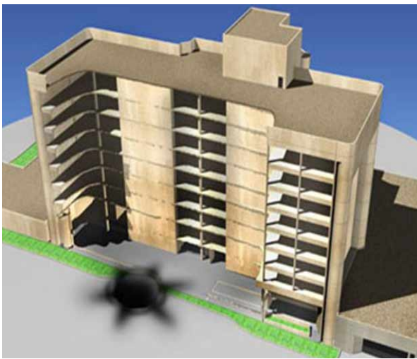
Figure 14 Estimated damage to internal shear wall on Line F in 1995 bombing scenario.
