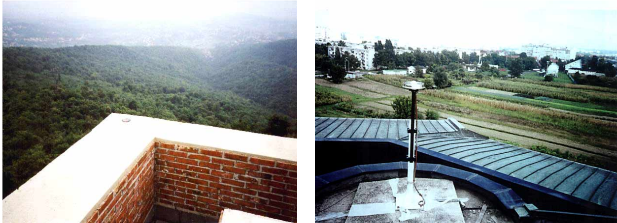
Fig.2. Marker of point 1036 at the Mt. Sljeme at Medvedgrad and antenna of the permanent GPS station Pt.1038
