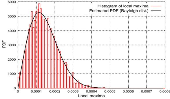
**Figure 8** Comparison of probability distributions for local maxima of response of 1DOF system at a specific time  $s_\ell = 300$ . The histogram is obtained from 5000-time MCS and the thin solid line is Rayleigh distribution calculated analytically.
