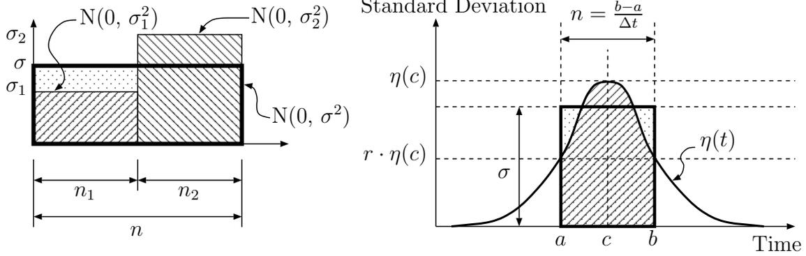
**Figure 4** Concept to replace i.n.n.i.d. Gaussian variable with i.i.d. Gaussian variable. **Figure 5** Concept to calculate the distribution of extreme value of non-stationary Gaussian white noise using the i.i.d. Gaussian variable.
