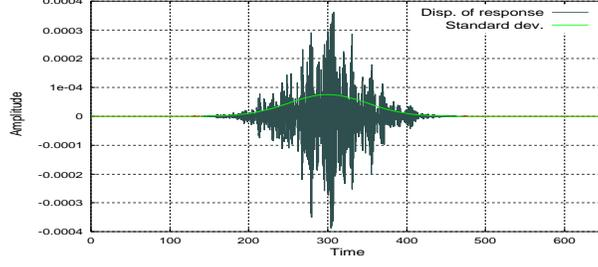
**Figure 7** An example of response function of 1DOF system ( $T_0 = 1$  and  $h = 0.05$ ) excited by the non-stationary Gaussian white noise shown in Figure 6. The smooth line shows the shape of Eq.(15) which is standard deviation of Rayleigh distribution estimated as the PDF for the local maxima.
