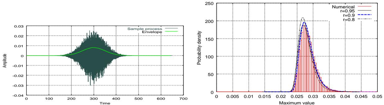
**Figure 6** An example of the approximate distribution for extreme values of non-stationary Gaussian white noise. The left panel shows a sample process and  $\eta(t) = \frac{1}{\sqrt{2\pi}50} \exp\left[-\frac{1}{2}\left(\frac{t-300}{50}\right)^2\right]$ . The approximate distributions for  $r = 0.95, 0.9,$  and  $0.8$  are compared with the result of numerical simulation in the right panel.
