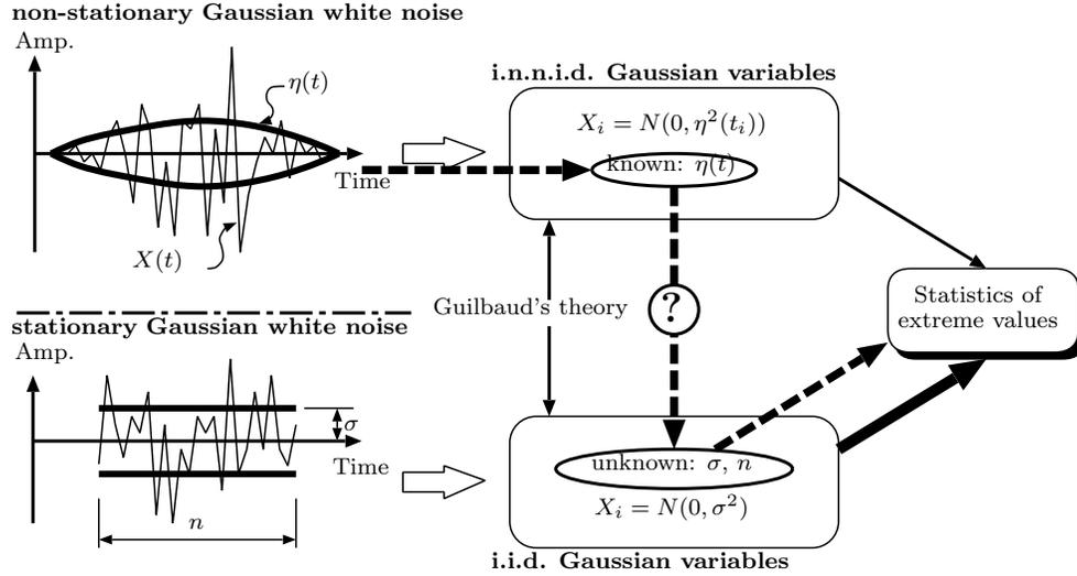
**Figure 1** Schematic diagram to show the relationship between i.n.n.i.d. and i.i.d. Gaussian variables and concept to derive the statistics of extreme values of non-stationary Gaussian white noise.
