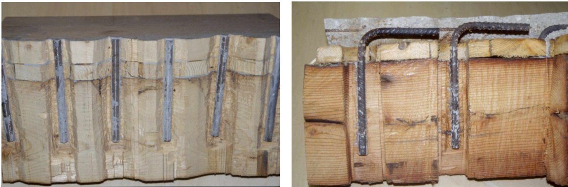
Figure 9. Glued-in steel connectors used for timber-based composite structures
