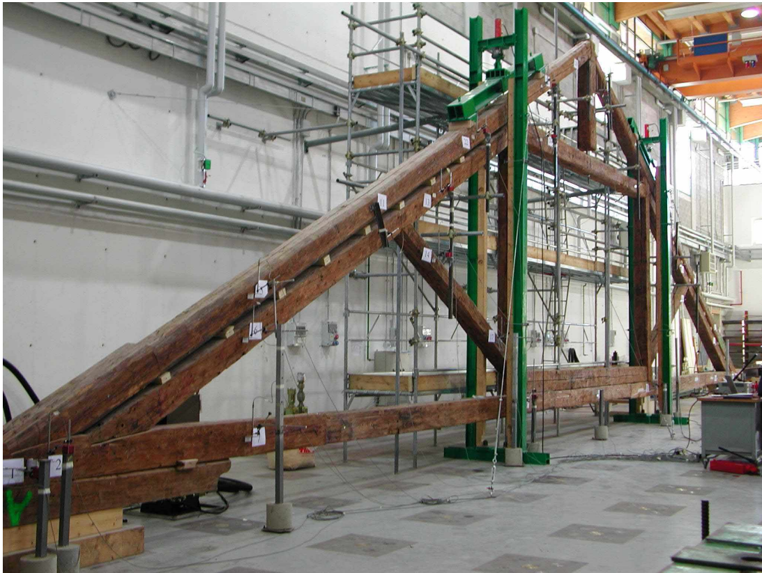
Figure 10. Experimental tests on the full scale model of a 25 m queen-post truss (Laboratory of the University of Trento)
