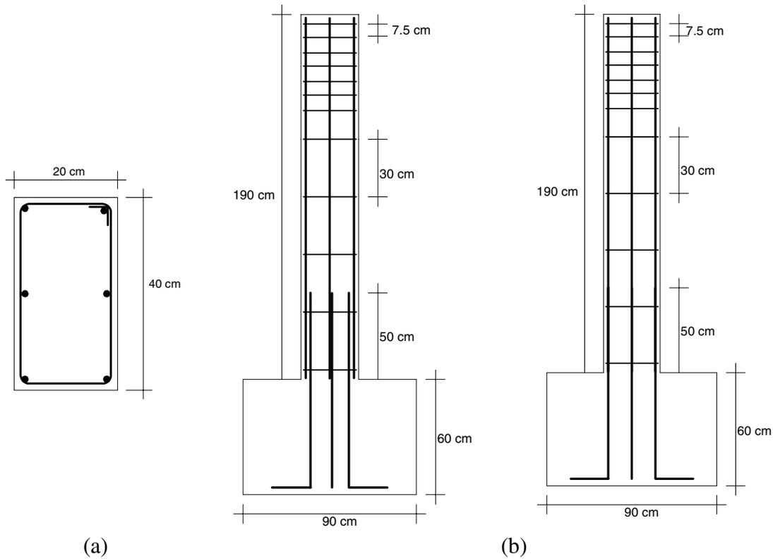
Figure 1. Details of test specimens
