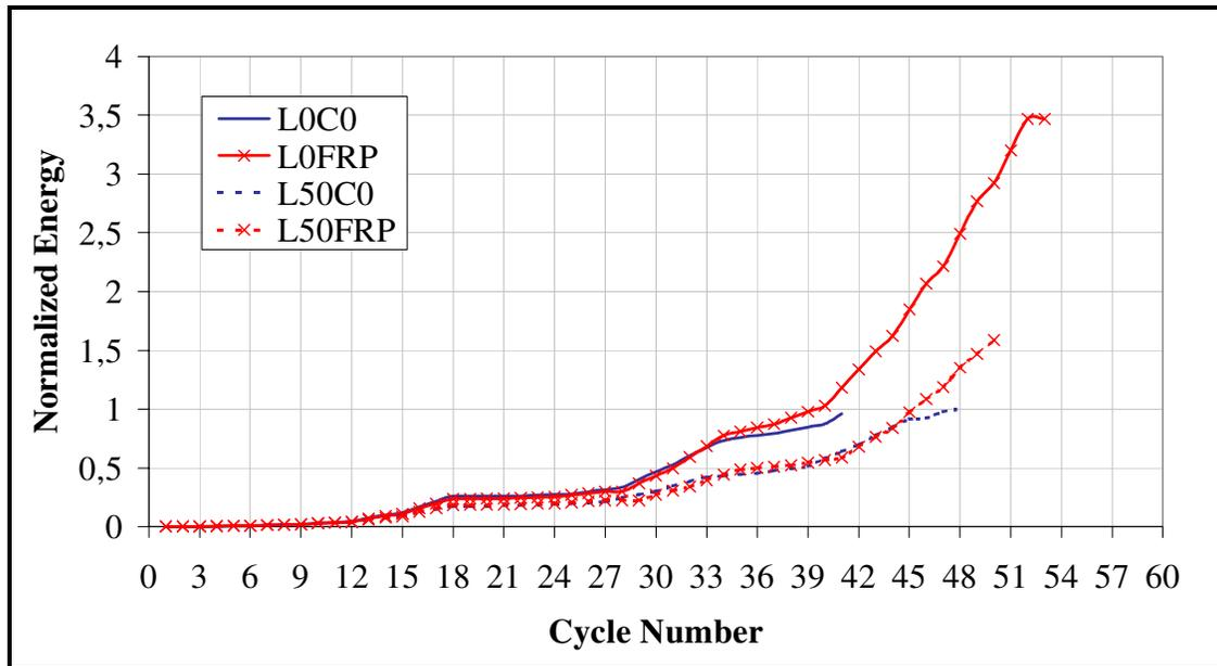
Figure 11. Energy dissipation of tested columns
