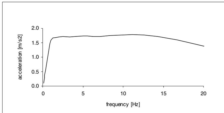
Figure 7 – Response spectrum of accelerations (RSA [8]) (Seismic Action n. 2, Soil type III (soft soil))
