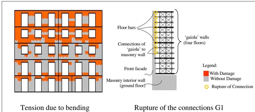
Figure 11 - Masonry damages and the rupture of connections at the end of the iterative process that allowed identifying the bending of the front façade collapse mechanism
