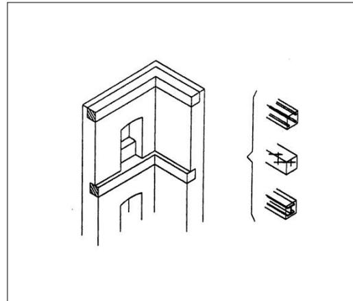
Figure 19 – More adequate strengthening solution (Croci [10])
