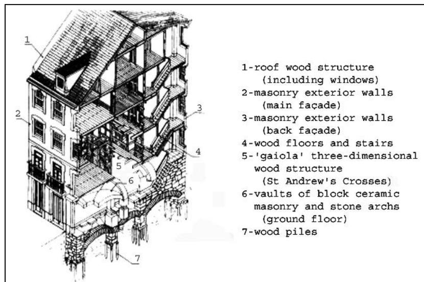
Fig. 1 – Structural details of a ‘Pombalino’ Building (*adapted from Mascarenhas [2]*)
