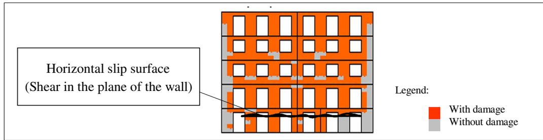
Figure 20 – Masonry shear damages identifying the shear base collapse mechanism ( $\gamma_{sis}=0.70$ )
