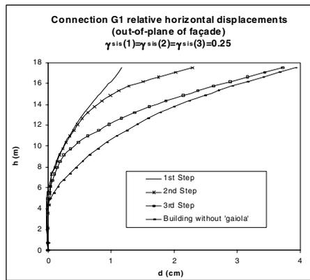
Figure 14- Horizontal displacements out-of-plane of the façade along the connection G1, relative to the corner of the building.
