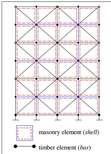
Figure 4 - Numerical model of a 'gaiola' wall panel (Cardoso [5])
