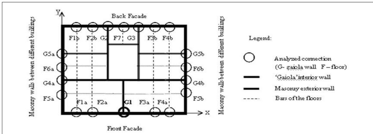
Figure 8 – Plan of the numerical model of the building identifying the different walls, the bars simulating the floors and the connections between the timber elements and the masonry walls
