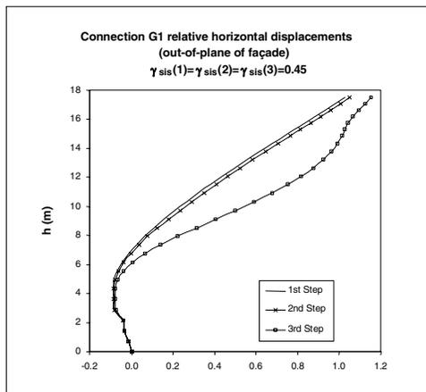
Figure 18 – Horizontal displacements out-of-plane of the façade after strengthening
