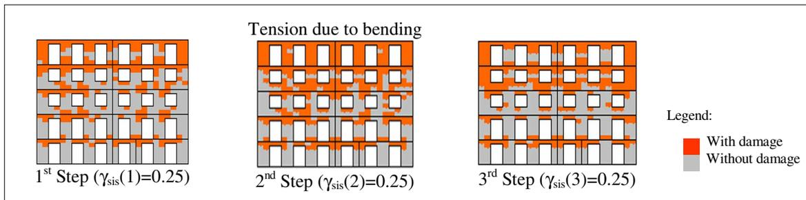
Figure 9 - Damage levels in masonry elements from main façade in iterative calculation
