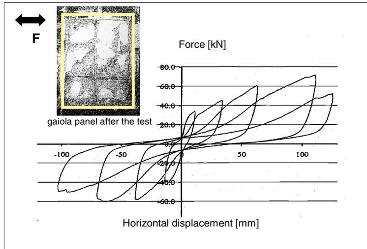
Figure 5 - Results of cyclic tests of a 'gaiola' wall panel removed from a 'Pombalino' building (Silva *et al.* [6])
