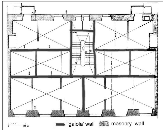
Figure 3 – Plan of a typical floor of the analyzed building (adapted from Santos [3])
