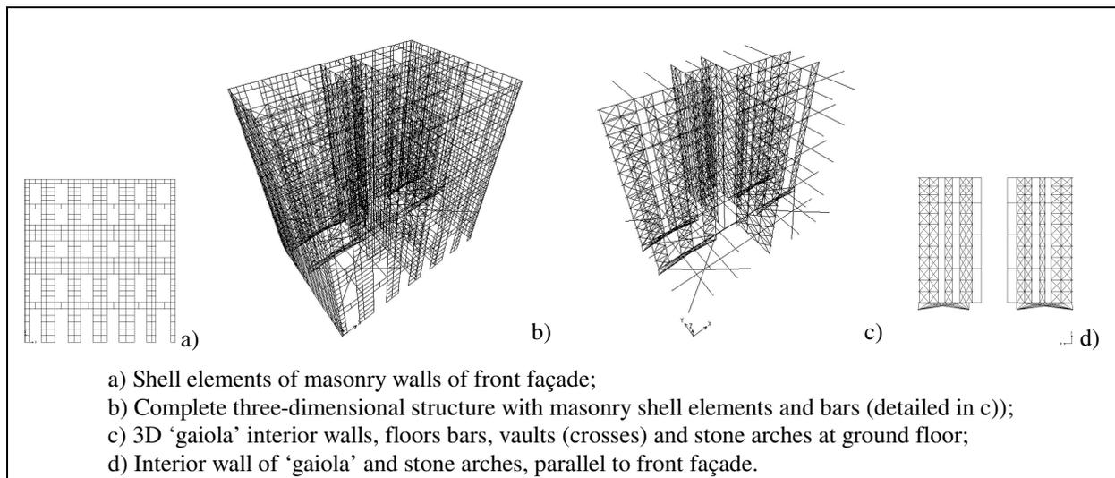
Figure 6 - Numerical model of the building (Cardoso [5])
