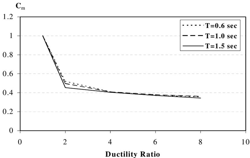
Figure 5. Effects of ductility ratio and period on the roof displacement factor,  $C_m$ , for 10-story models
