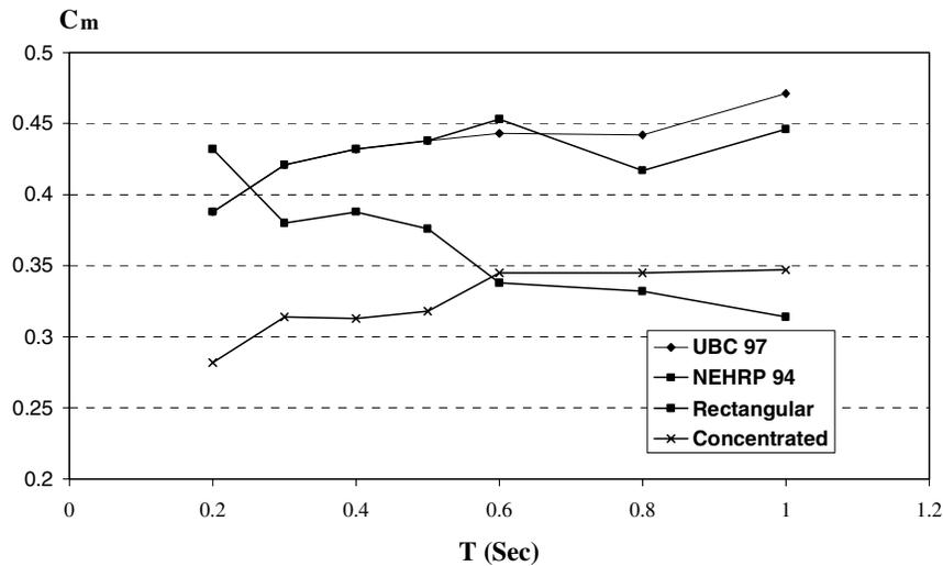
Figure 4. Effect of different distribution patterns of seismic load on  $C_m$  for 5-story models with  $\mu=6$
