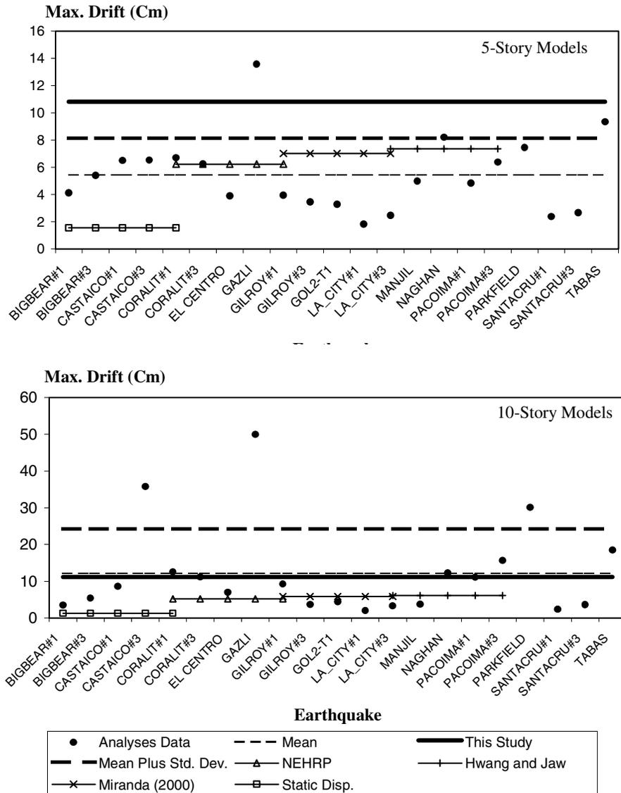
**Figure 8. A comparison between the dynamic analyses results and the maximum inter-story drift as proposed by NEHRP, Hwang and Jaw, Miranda and this study for the 5 and 10-story moment-resisting frames**
