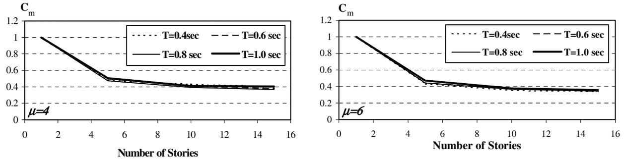
Figure 6. Effect of the number of stories on the roof displacement factor,  $C_m$ , for  $\mu=4$  and 6
