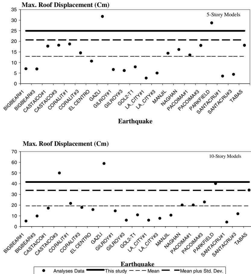
**Figure 9. A comparison between the dynamic analyses results and the maximum roof displacement as proposed by this study for the 5 and 10-story moment-resisting frames**
