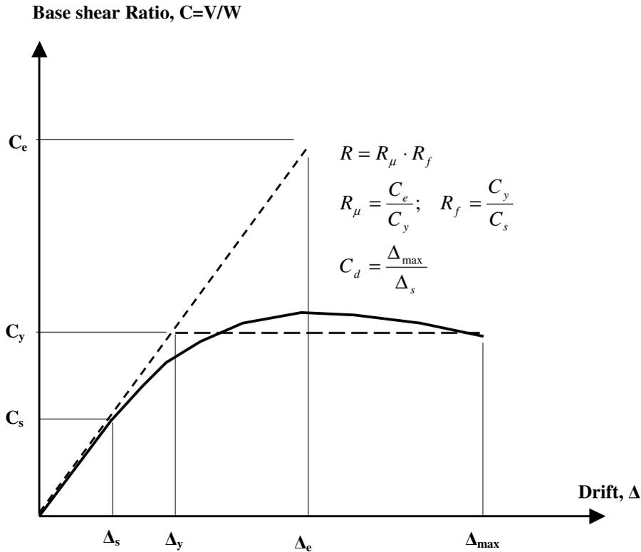
**Figure 1. Effect of Inelastic Behavior on Seismic Response**
