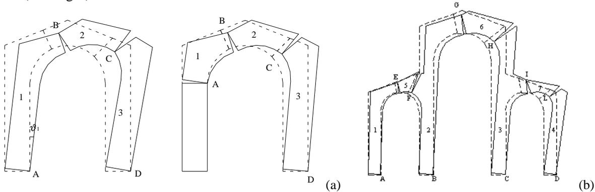
**Figure 7. Possible kinematisms in triumphal arches: (a) single-nave church; (b) three-nave church.**
