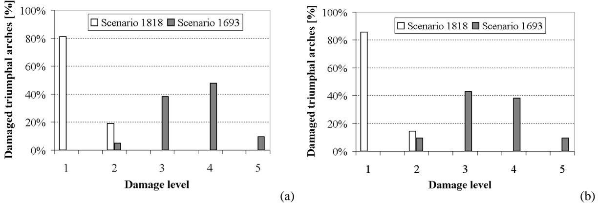
**Figure 9. Damage scenarios for triumphal arches: (a) without the tie-rod; (b) with the tie-rod.**
