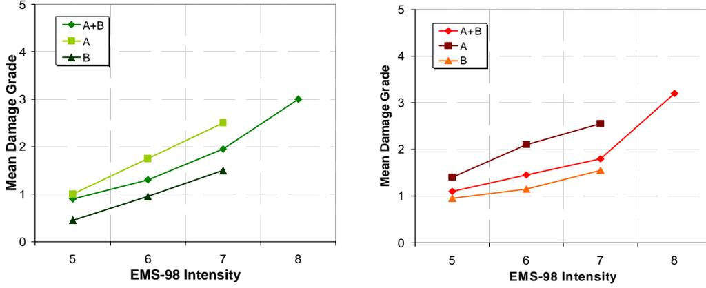
**Figure 2. Mean damage grade of Umbria and The Marches churches.**
