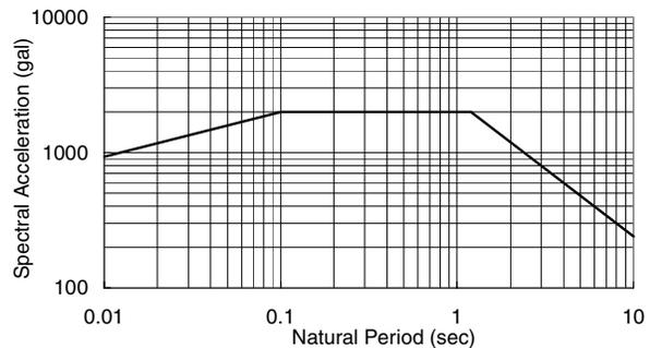
Figure 10: Acceleration Response Spectrum
