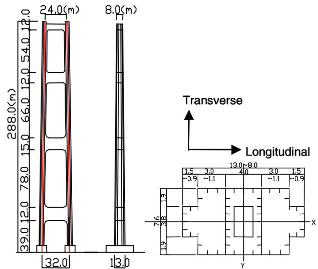
Figure 1: Tower Elevation and Cross-Section
