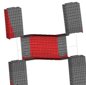
**Figure 8: Shear Damage of Beam**
