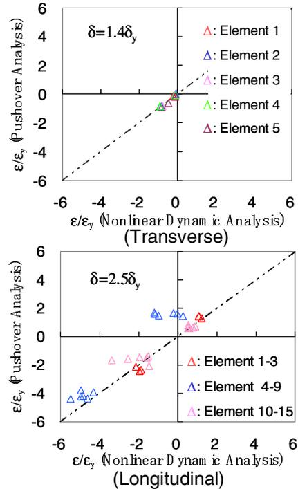
**Figure 12: Comparisons of Strain Ratio**
