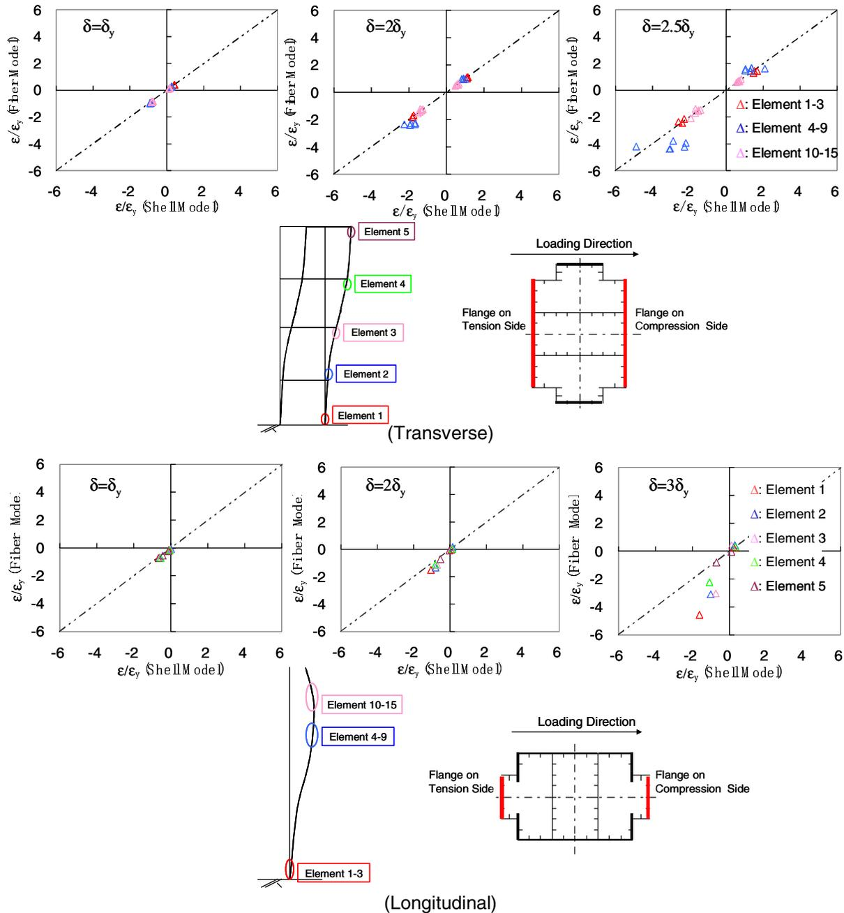
**Figure 7: Comparisons of Strain Ratio**
