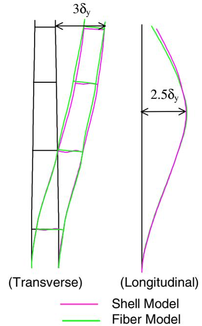
**Figure 5: Comparisons of Deformed Tower Shapes**
