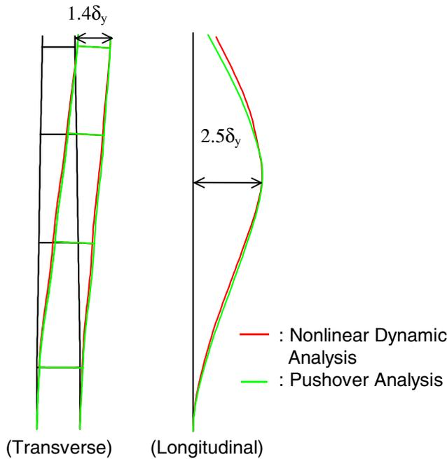
**Figure 11: Comparisons of Deformed Tower Shapes**
