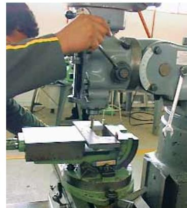
(b) final smoothing of the internal edge of the C-plate
