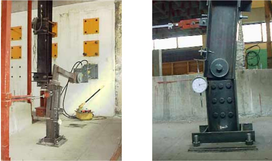
Figure 5. Cyclic testing of an individual rotational friction device
