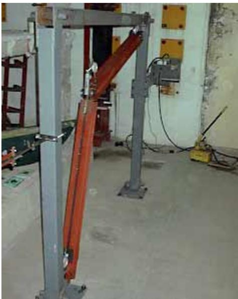
(a) frictional bracing installed into a steel frame with pinned connections
