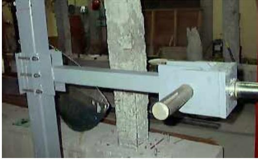
(a) pinned strut connected to south column
