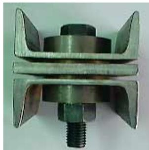
Figure 8. Transverse view of the rotational friction device installed in the dissipative bracing
