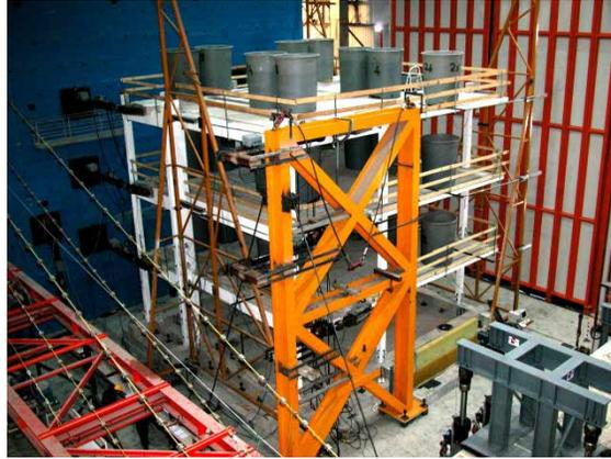
**Figure 4 – The SPEAR structure before the first round of PsD tests**
