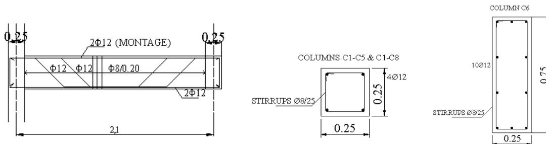
Figure 2 – Details of the beam and column rebars
