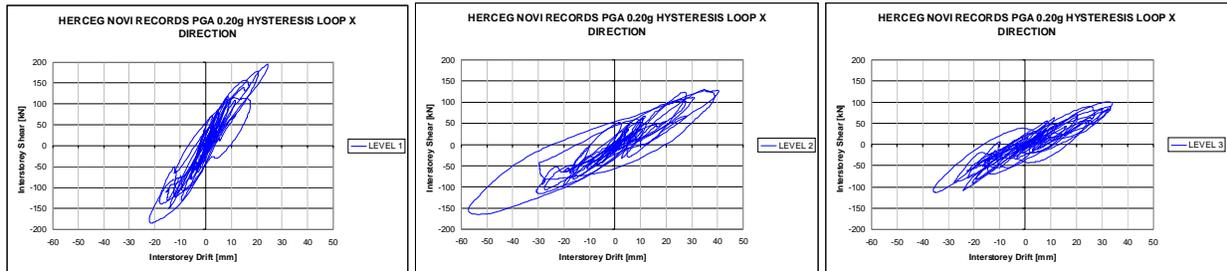
**Figure 13 – Hysteresis loops in the X direction**
