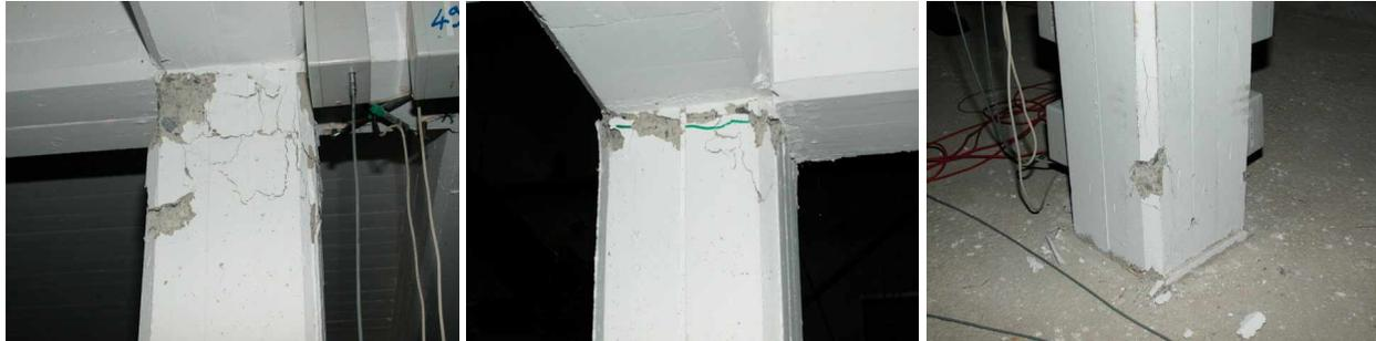
**Figure 21 – Damage after the 0.2g PGA test: a) extensive spalling at the top of columns (C3); b) light spalling and flexural cracking at the top of corner columns (C1); c) base of column C3**
