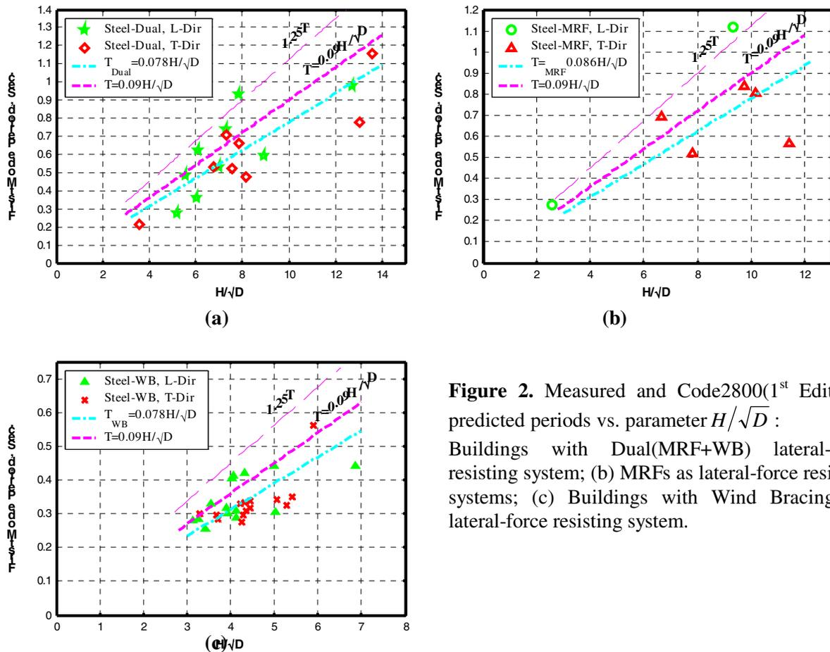
**Figure 2.** Measured and Code2800(1<sup>st</sup> Edition)-predicted periods vs. parameter  $H/\sqrt{D}$  : (a) Buildings with Dual(MRF+WB) lateral-force resisting system; (b) MRFs as lateral-force resisting systems; (c) Buildings with Wind Bracings as lateral-force resisting system.
