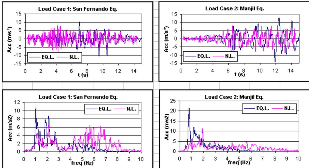
Figure 10: Crest acceleration time histories and their Fourier amplitude spectra in EQL and NL analyses for two load cases.
