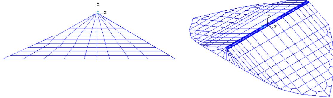
**Figure 8: Three dimensional finite element model of the dam (maximum section and isometric view)**
