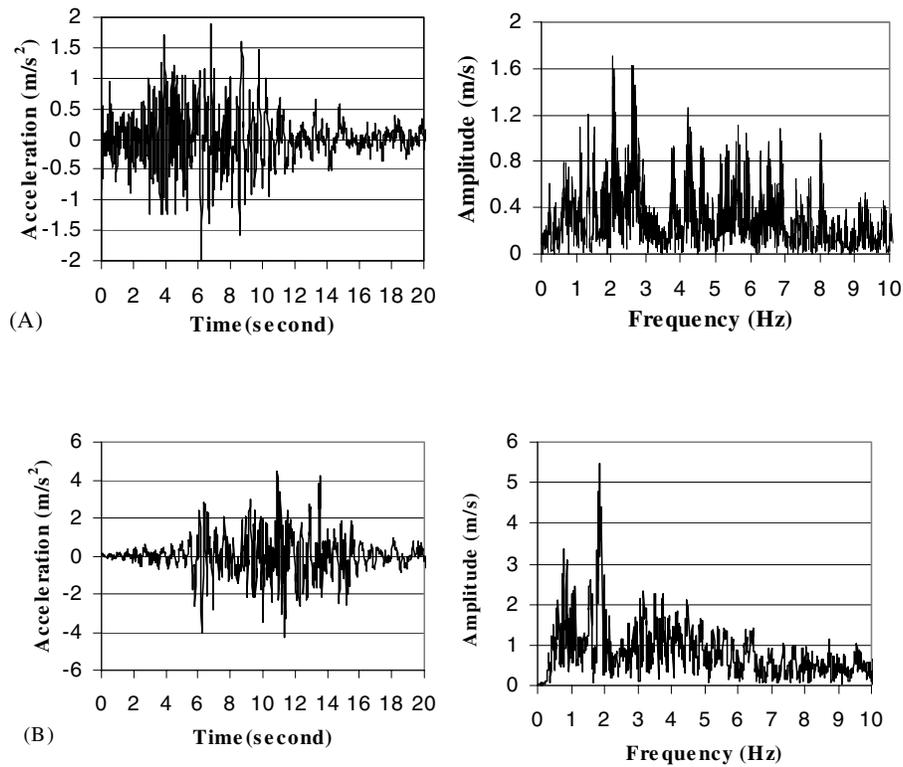
**Figure 9: Dynamic characteristics of two excitations used in numerical analyses: (A) NS component of San Fernando Eq. - load case 1; (B) L component of Manjil – Iran Eq. - load case 2**
