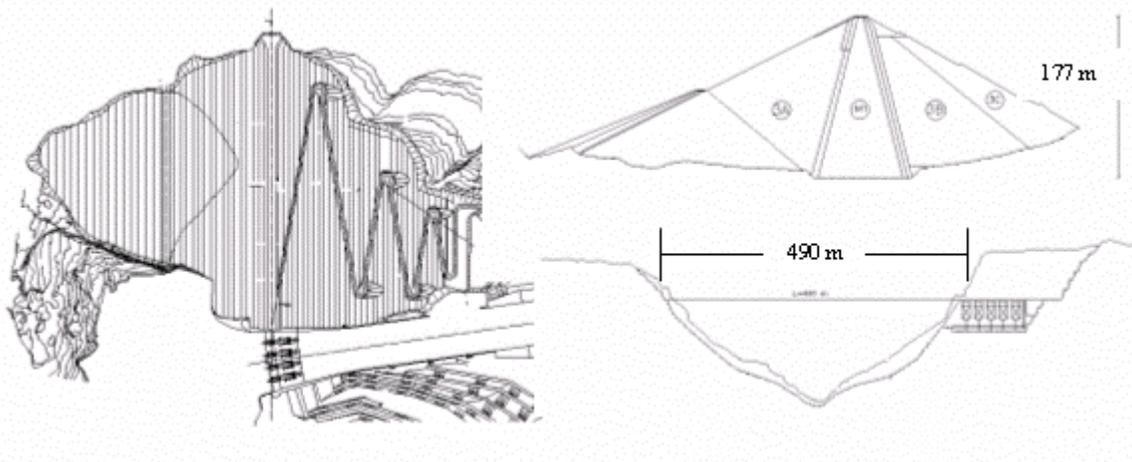
**Figure 1: Plan view, maximum and longitudinal section of Masjed-Soleyman dam**
