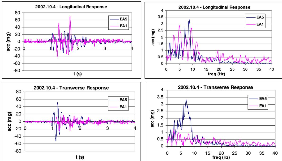
**Figure 5: Time and frequency history of dam recorded at two locations (crest: EA1 and dog way: EA5) during seismic excitation on 2002.10.4, in longitudinal and transverse directions**
