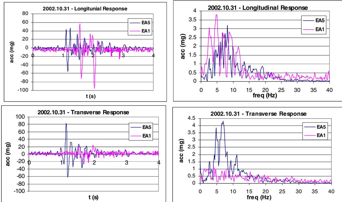
**Figure 7: Time and frequency history of dam recorded at two locations (crest: *EAI* and dog way: *EA5*) during seismic excitation on 2002.10.31, in longitudinal and transverse directions**
