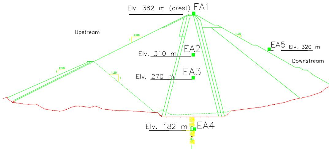
**Figure 4: Maximum dam cross section and location of deployed accelerometers in and on this section (Ch. 260 m)**
