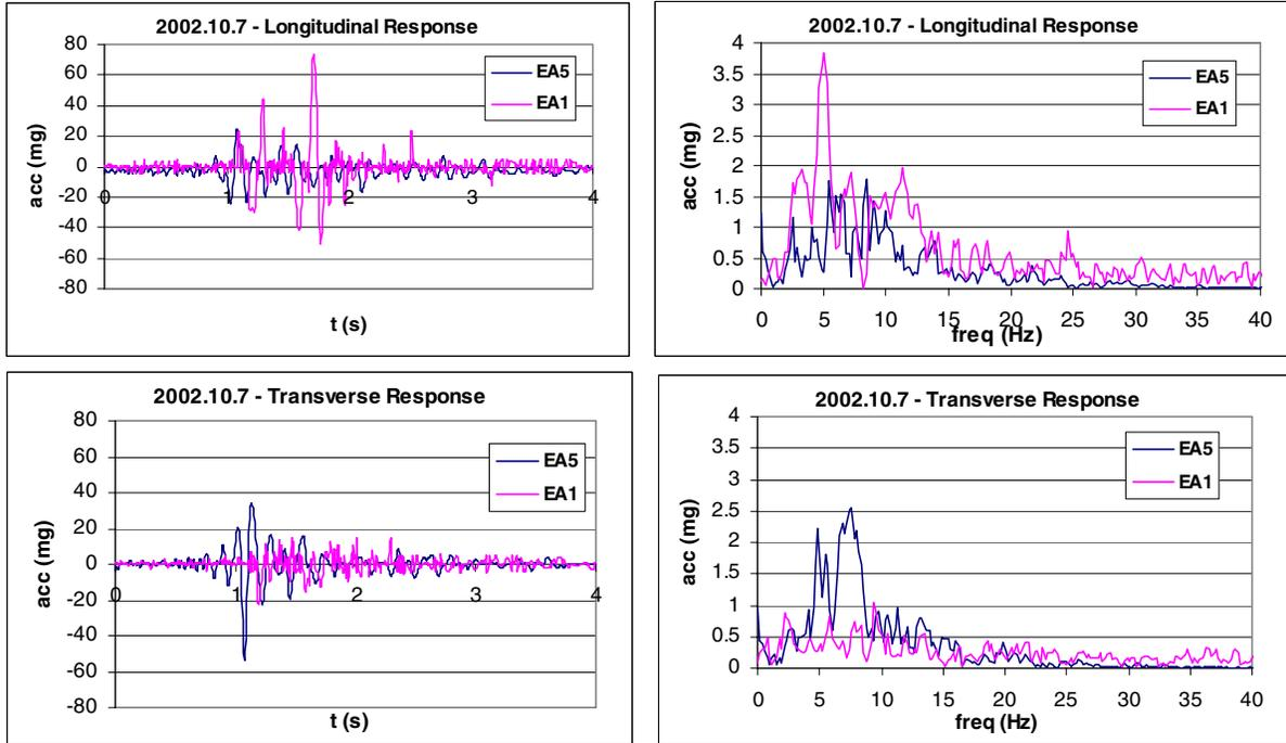
Figure 6: Time and frequency history of dam recorded at two locations (crest: EA1 and dog way: EA5) during seismic excitation on 2002.10.7, in longitudinal and transverse directions
