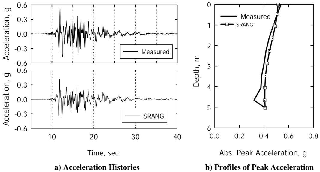
**Fig. 3 Measured and Computed Acceleration Responses of Dry Sand Layer**
