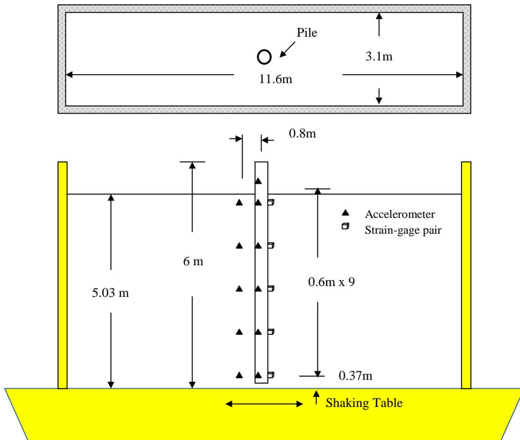
**Fig. 1 Large-Scale Shaking-Table Test Set-up**
