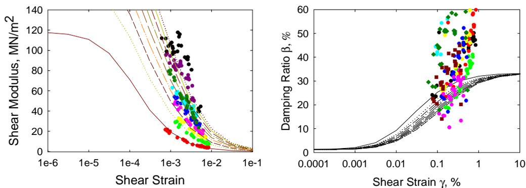
**Fig. 2 Shear Moduli and Damping Ratios from Large-Scale Tests**
