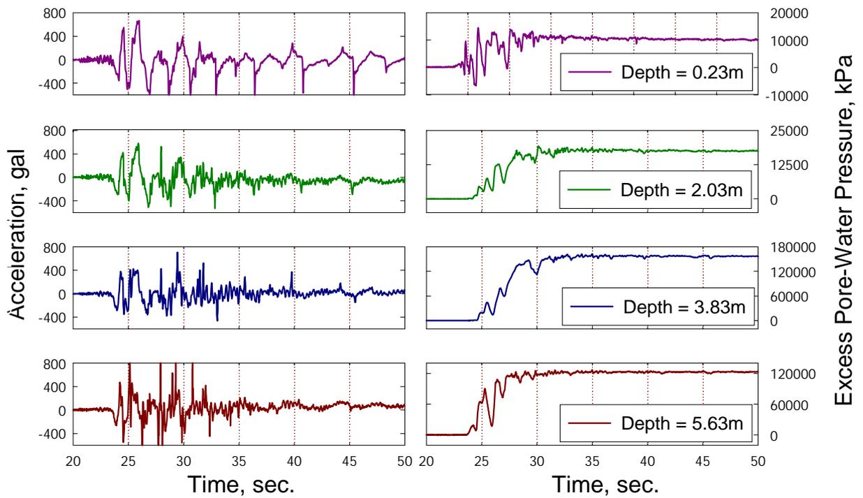
**Fig. 4 Measured Responses of Saturated Sand Layer in Large-Scale Test**
