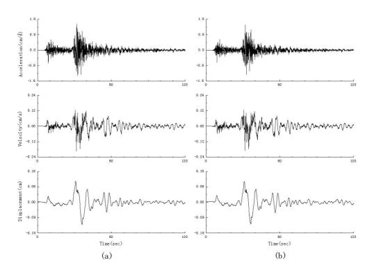
Fig. 2 Recovered ground acceleration, velocity and displacement (from top to bottom, respectively) from VBB and LG of BJI station (a) VBB (b) LG
