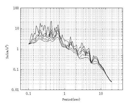
Figure 5 The absolute acceleration response spectra from E-W component of VBB of BJI for Zhangbei earthquake. From top to bottom  $\zeta$ =0, 0.01, 0.02, 0.05, 0.10
