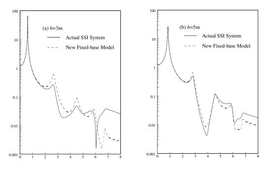
Figure 2. Comparison of roof floor displacement in the frequency domain
