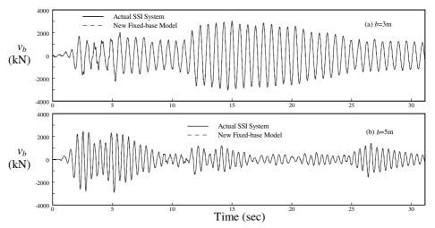
Figure 3. Comparison of base shear to El Centro earthquake
