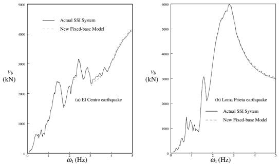
Figure 5. Comparison of base shear spectrum to different earthquakes
