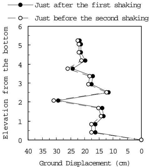
Figure 14: Displacement of liquefied ground without shaking
