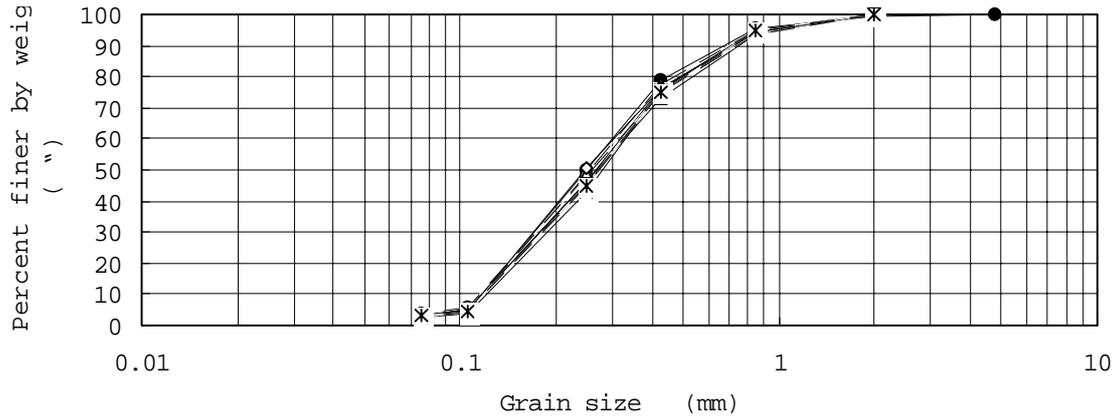
**Figure 1: Grain size distribution curves of tested sand**
