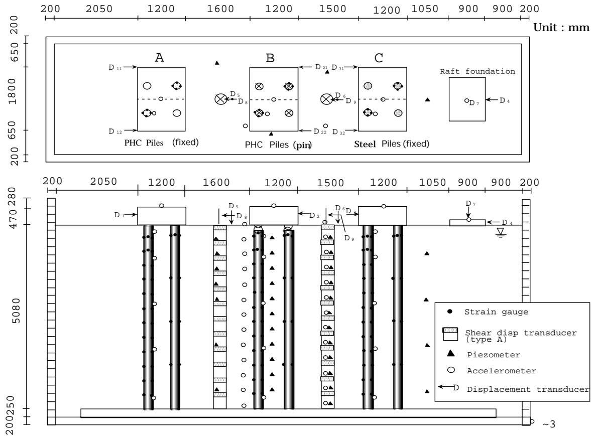
Figure 3: Schematic diagram of the ground, pile foundations and sensors in the first test
