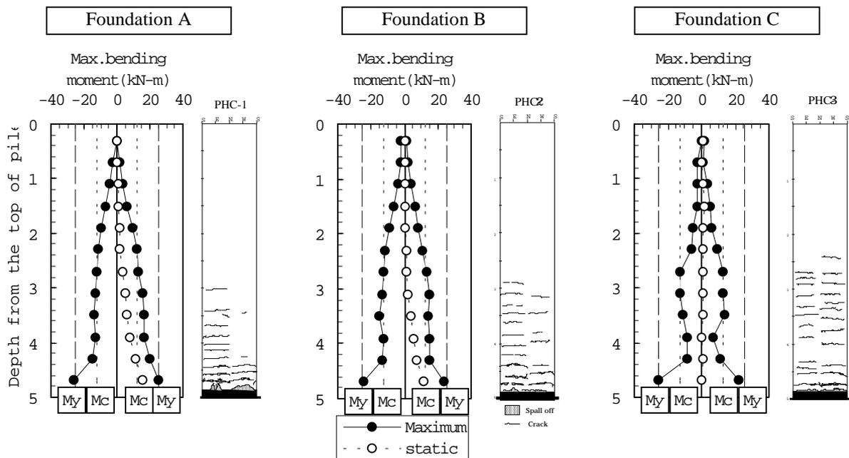
**Figure 16: Measured maximum bending moments and observed cracks on PHC piles**
