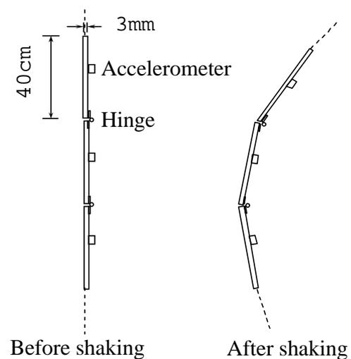
Figure 7: Schematic diagram of shear displacement sensor (Type B)
