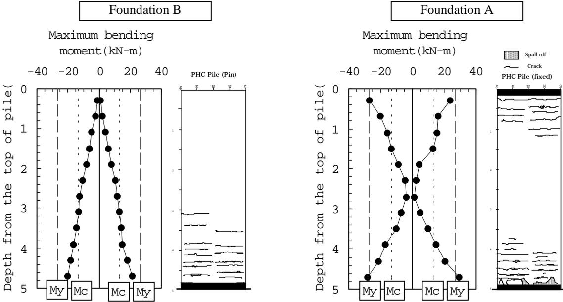
Figure 11: Measured maximum moments and observed cracks on PHC piles
