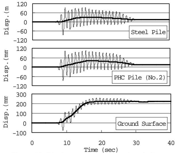
Figure 15: Displacement time histories of pile tops and ground surface
