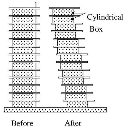
Figure 5: Schematic diagram of shear displacement transducer (Type A)
