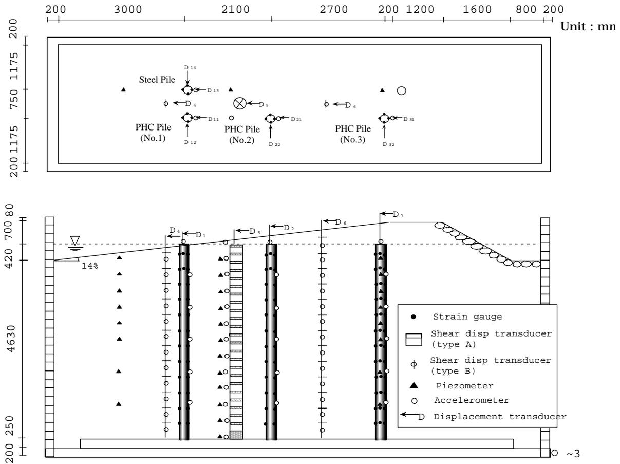
Figure 6: Schematic diagram of the ground, pile foundations and sensors in the second test
