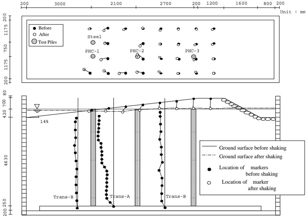
Figure 13: Displacement distribution on the ground measured after the first step of shaking
