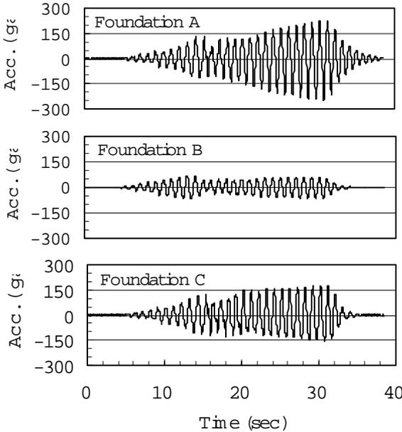
**Figure 9: Time histories of footing accelerations under 150gals of shaking**
