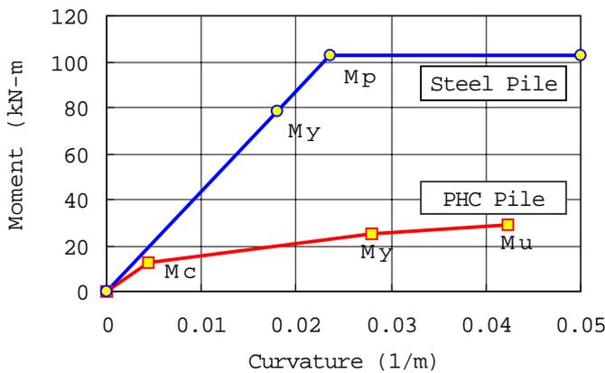
Figure 4: Relation between bending moment and curvature of piles tested
