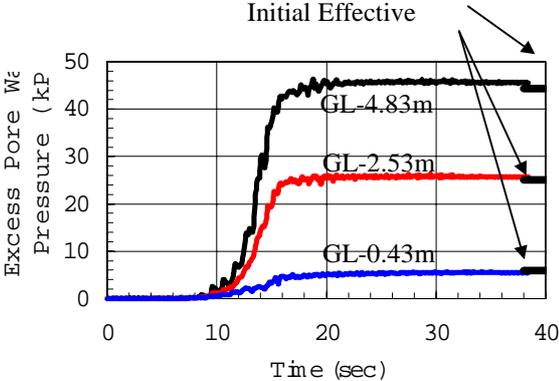
**Figure 8: Time histories of excess pore water pressure ratio**
