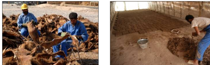
Figure 10 Process of producing the reinforced adobes with the palm fibers
