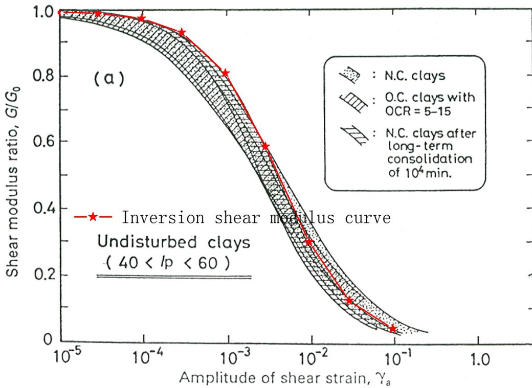
Fig. 5 Inversion shear modulus curve of clay in TKCH07 site
