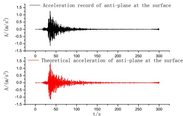
Fig.7 Theoretical value and the actual observations of the surface at TKCH07 site in M<sub>7.1</sub> earthquake
