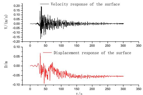
Fig.8 Theoretical velocity and displacement history of the surface at TKCH07 site in M<sub>7.1</sub> earthquake
