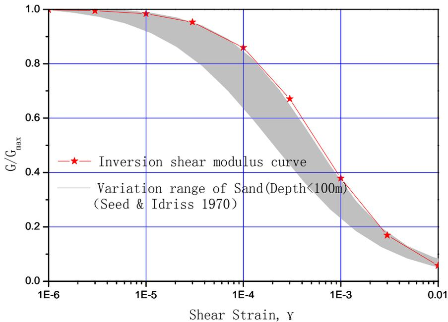
Fig. 3 Inversion shear modulus results of sand in TKCH07 site
