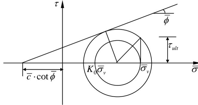
Fig.1 Ultimate shear stress  $\tau_{ult}$
