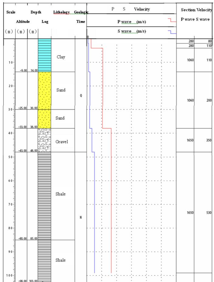
Fig.2 Soil and rock condition of TKCH07 site
