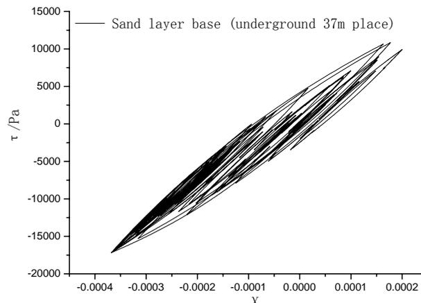
Fig.9 Inversion nonlinear hysteretic constitutive relations in time domain at the bottom of sand layer(underground 37m place) in  $M_j7.1$  earthquake
