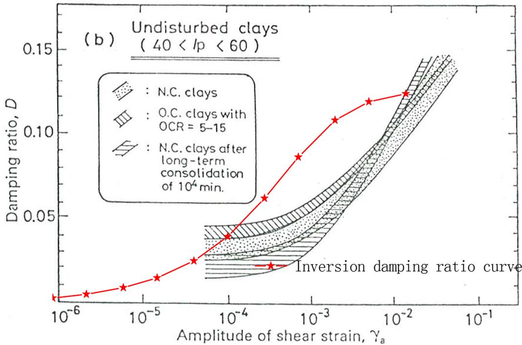
Fig.6 Inversion damping ratio curve of clay in in TKCH07 site
