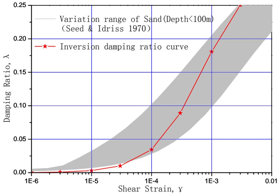
Fig. 4 Inversion damping ratio of sand in TKCH07 site
