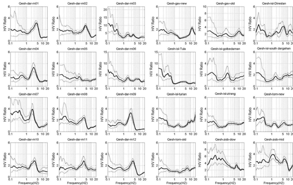
Figure 9. Amplification curves obtained by Microtremors in the Dargahan (3 left column) and the other stations across the Island (3 right column).
