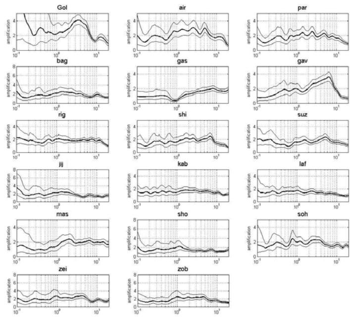
Figure 5. Amplification ratios obtained using HVSR method for all stations
