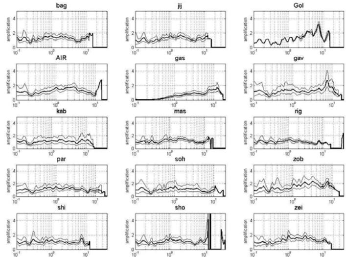
Figure 6. Amplification ratios obtained using SSR method for different stations
