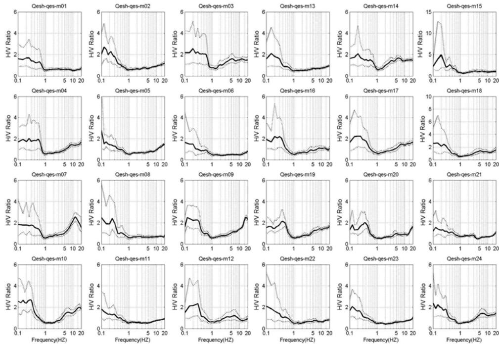
Figure 8. Amplification curves obtained by Microtremors in the Qeshm city.
