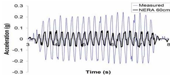
Figure 5 Comparison with NERA and Measured acceleration of loose model at 60 cm.
