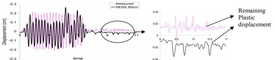
Figure 9. Comparison with NERA and Measured displacement of loose model.
