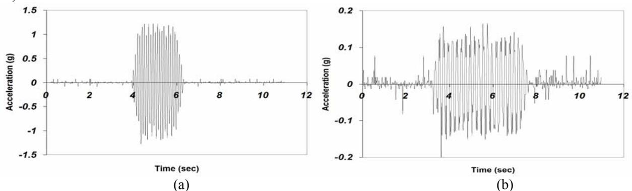
Figure 2 Input excitation of (a) dense (b) loose sand.
