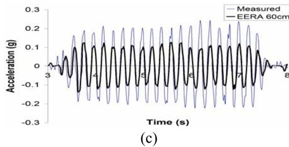
Figure 4 Comparison with EERA and Measured acceleration of loose model at (a) 20 cm (b) 40 cm and (c) 60 cm.
