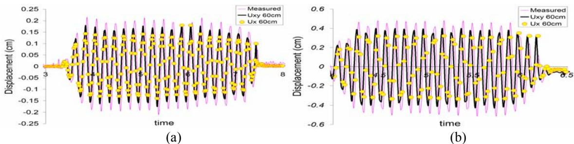
Figure 13 Comparison with  $U_x$ ,  $U_{xy}$  and Measured displacement of (a) loose (b) dense models at 60 cm.
