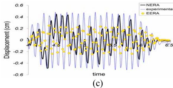
Figure 10 Comparison of EERA, NERA and Measured displacements in dense model at (a) 20 cm (b) 40 cm and (c) 60 cm.
