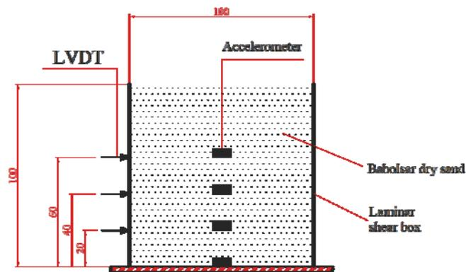
Figure 1 Configuration of instruments in laminar shear box (dimensions are in  $cm$ ).
