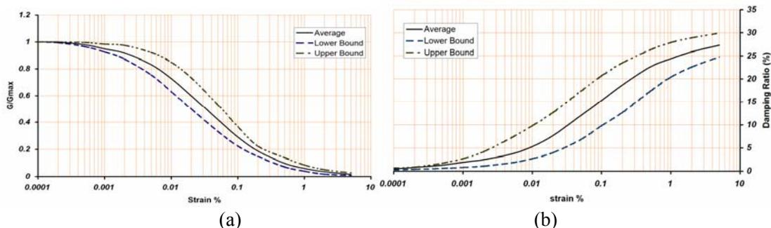
Figure 3 Curves of (a)  $G/G_{max}$ - $\gamma$ ; (b) Damping Ratio(%)- $\gamma$  at 0.0001% - 10% strain (Seed and Idriss, 1970)
