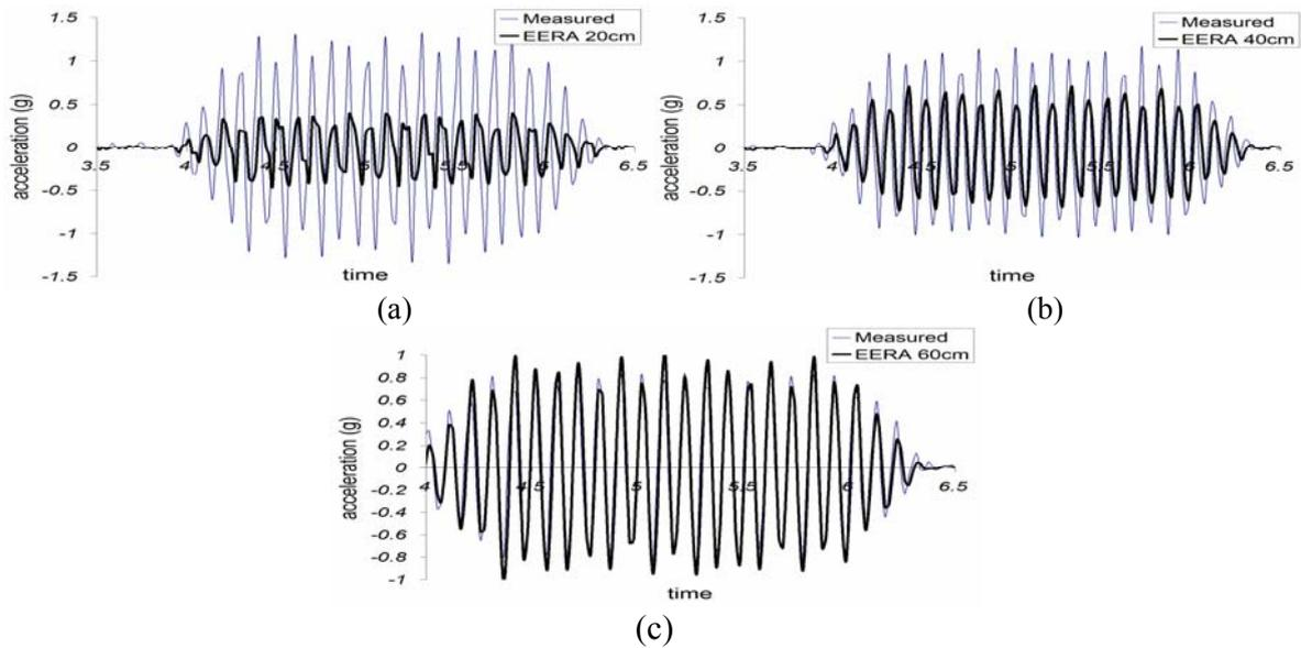
Figure 6 Comparison with EERA and Measured acceleration of dense model at (a) 20 cm (b) 40 cm and (c) 60 cm.
