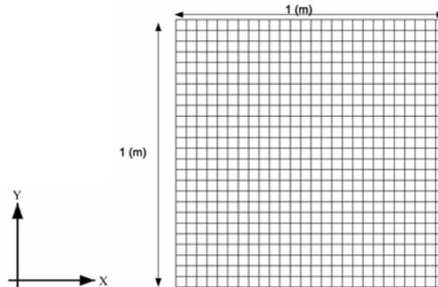
Figure 11 2D finite element mesh of laminar shear box.
