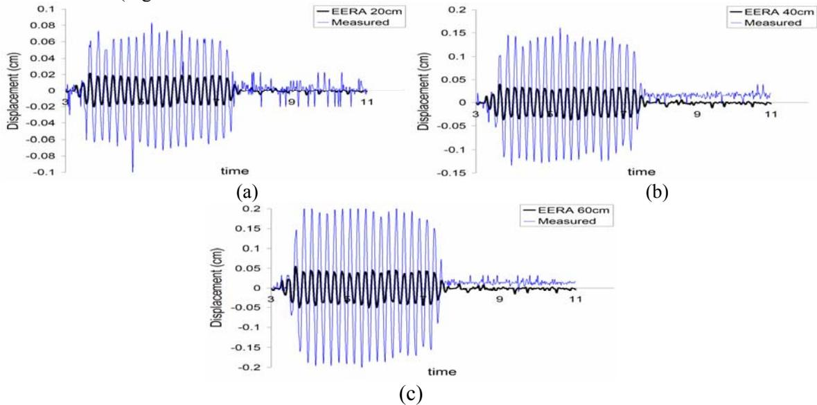
Figure 8 Comparison with EERA and Measured displacement of loose model at (a) 20 cm (b) 40 cm and (c) 60 cm.
