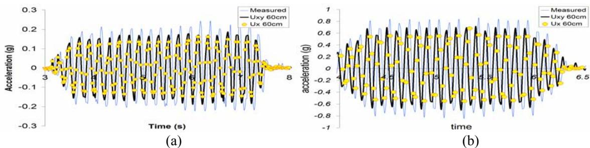
Figure 12 Comparison with  $U_x$ ,  $U_{xy}$  and Measured acceleration of (a) loose (b) dense models at 60 cm.
