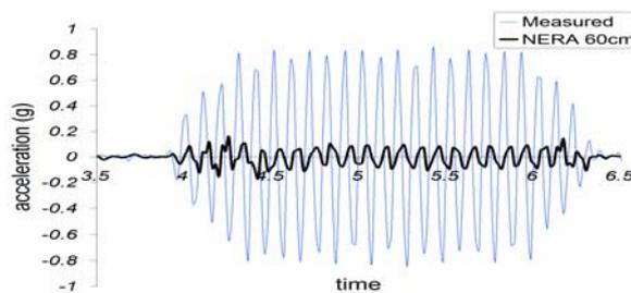
Figure 7 Comparison with NERA and Measured acceleration of dense model at 60 cm.
