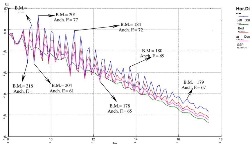
Figure 8 Disp. of different points and some bending moment (t-m/m) and anchor forces (t/m) during earthquake
