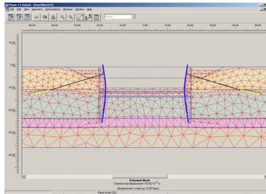
Figure 7 Deformed mesh after excavation and dock floor construction (scaled to 15 times greater)
