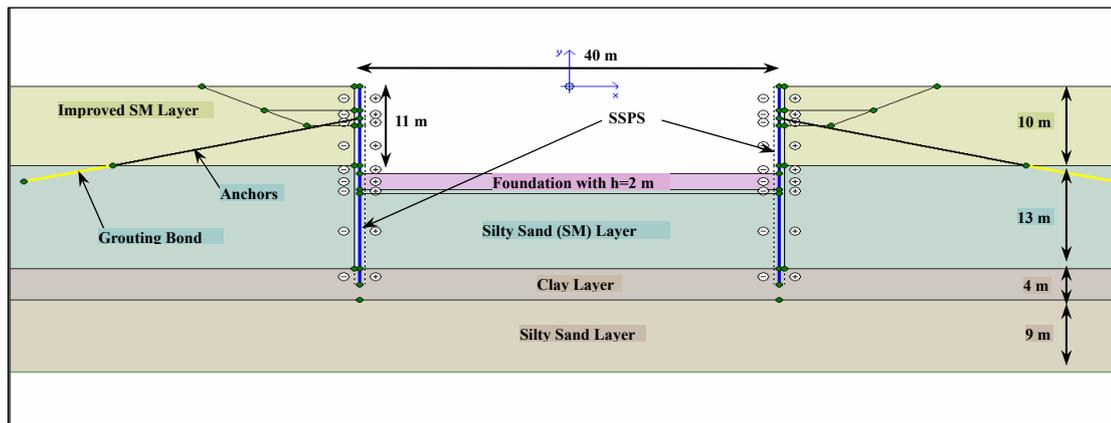
Figure 2 Dry dock geometry and soil stratification
