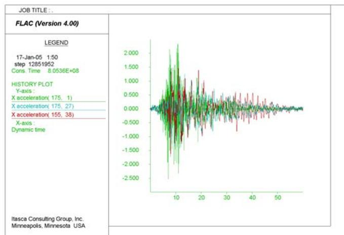
Figure 9 Recorded acceleration time history in three points of bedrock, dock floor and top of SSP
