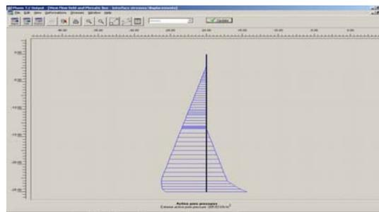
Figure 6 Unbalance water pressure on a sheet pile after seepage analysis
