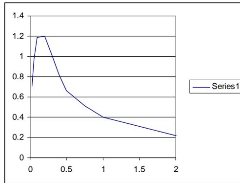
Figure 2- Uniform response spectrum of Maku dam site in the Maximum Design Level
