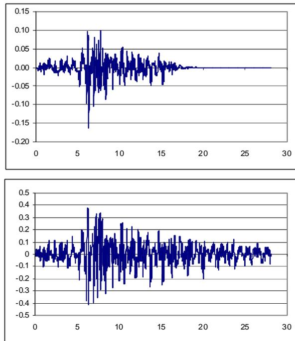
Figure 4- Initial and final Chaldiran 1976 acceleration time histories before and after spectral matching to the target spectrum.
