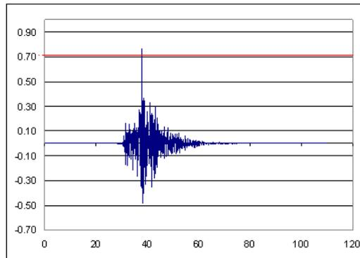
Figure 3- Acceleration time history of 2006.9.5 earthquake after spectral matching with target spectra. Red line shows the critical acceleration to yield slides in Maku dam site.
