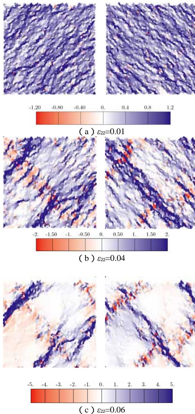
Left slip deformation      Right slip deformation
