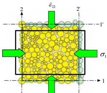
Figure 2 Biaxial compression test of granular materials with periodic boundaries
