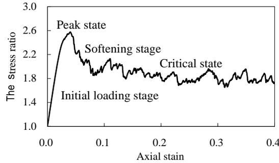
Figure 3 The stress ratio versus axial strain
